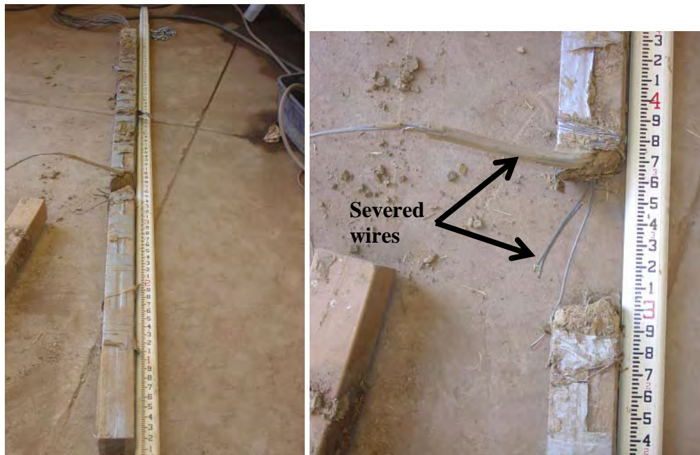
Figure 6.30 Photographs of member IM-18 after excavation: (a) complete member and (b) close up of the failure surface.
