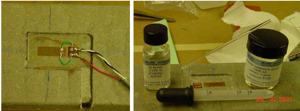
Figure 5.2 Photographs of 350-Ohm electrical resistance strain gages used to monitor strains in the recycled plastic reinforcing members.
