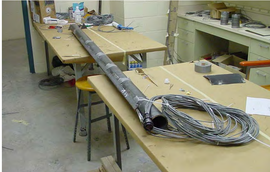
Figure 5.4 Photograph of instrumented steel pipe member with 0.5-in angle section to protect gages during installation.
