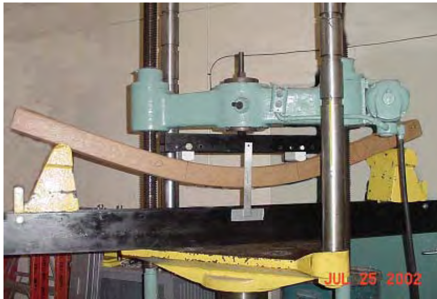
Figure 3.18 Photograph of four-point flexure test in progress.
