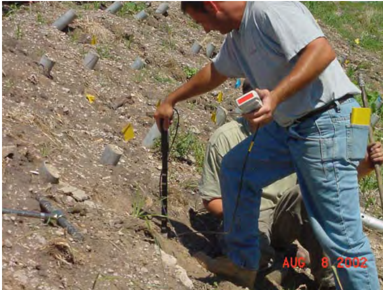
Figure 5.14 Photograph of Profile Probe ® while taking readings.
