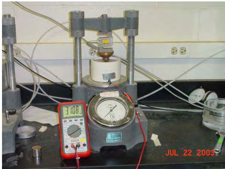
Figure 5.8 Apparatus used to develop calibration for FSR.
