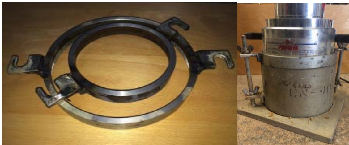
Figure 4-14. Attached collar during LWD on mold testing
