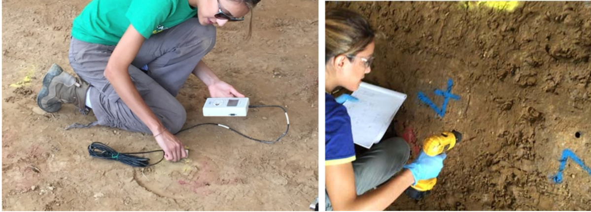
Figure 3-10. Decagon GS-1 VWC sensor inserted from the top on the ALF soil; VWC reading with ProCheck; Using a drill to prefabricate holes for the Decagon GS-1 VWC sensor insertion into HPC soil
