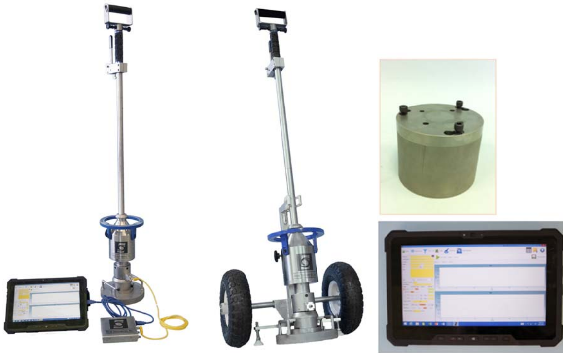
Figure 2-8. Olson LWD-01 with the new ruggedized DELL tablet and optional lighter (~8.5 lbs) drop weight (pictures courtesy of Olson Engineering Inc.)
