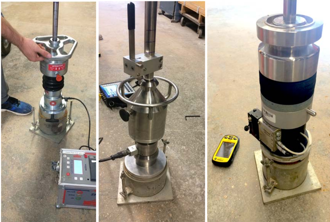
Figure 3-37. Configuration of Zorn, Olson, and Dynatest LWDs on top of the Proctor mold
