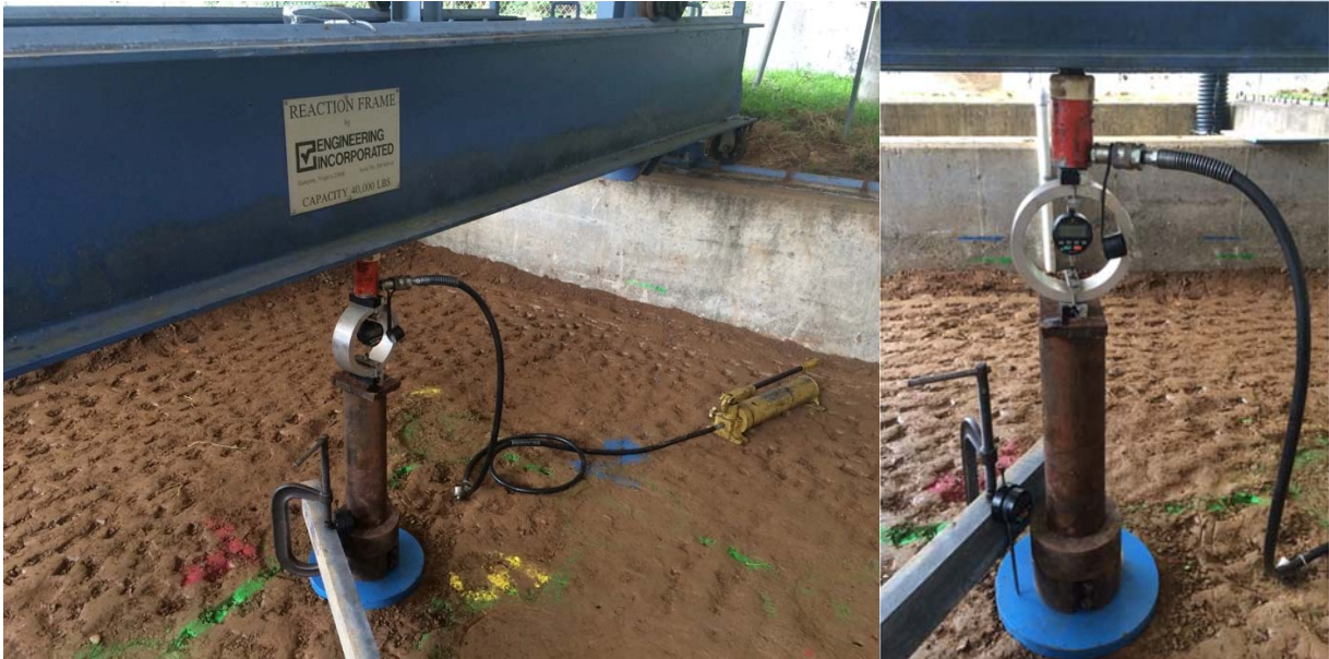
Figure 3-25. Static plate load test on the test pit
