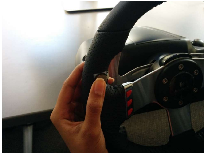
Figure 4: A Pressure Sensor Deployed on a Logitech G27 Racing Wheel Controller
