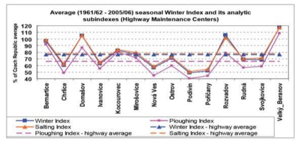
Graphical representation of performance measurement indices used in the Czech Republic. (PIARC, 2015)
