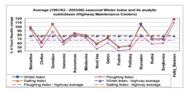
Figure A.5.2 Graphical representation of performance measurement indices used in the Czech Republic (adopted from PIARC 2015)
