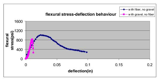
Figure 13. The effect of fiber on flexural stress against that of gravel
