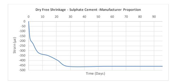
Figure 14. Shrinkage strain Vs Time: Sulfate cement with manufacturer mix proportion
