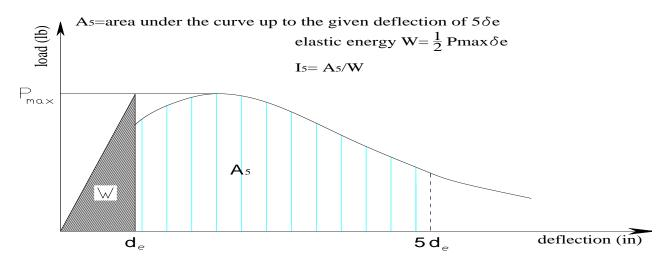
Figure 23. Graph for toughness index Is
