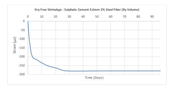
Figure 16. Shrinkage strain Vs Time: Sulfate cement with 2% steel fibers
