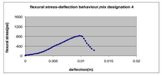
Figure 7. Flexural Stress-Deflection Behavior for Sample #4
