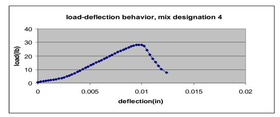
Figure 5. Load-deflection Behavior for Sample #4
