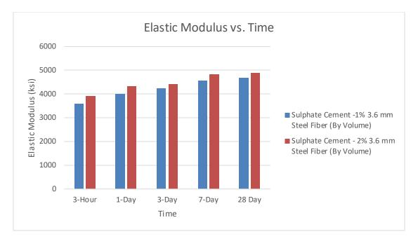
Figure 22. Elastic Modulus based on compressive tests
