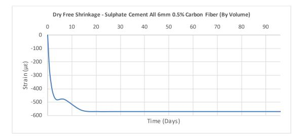
Figure 17. Shrinkage strain Vs Time: Sulfate cement with 0.5% carbon fibers
