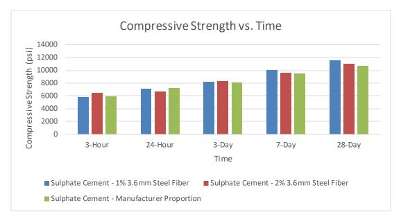
Figure 21. Compressive Strength tests
