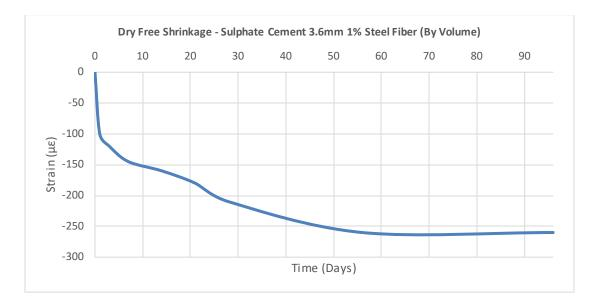
Figure 15. Shrinkage strain Vs Time: Sulfate cement with 1% steel fibers
