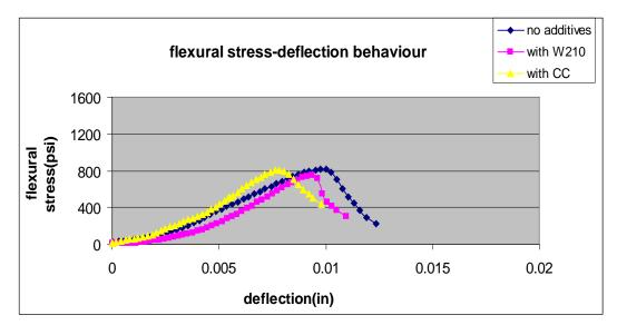
Figure 9. Influence of Alumino-silicates on modulus of rupture: samples without gravel
