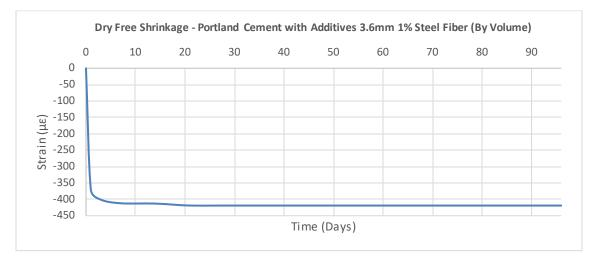
Figure 19. Shrinkage strain Vs Time: Portland cement with additives, 1% steel fibers
