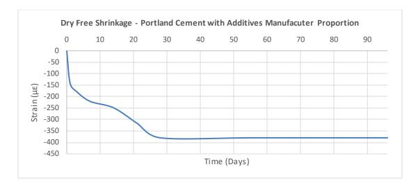
Figure 18. Shrinkage strain Vs Time: Portland cement with additives, Manufacturer recommended mix proportion
