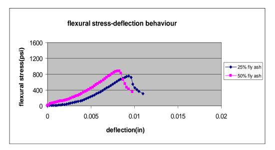
Figure 8. Influence of Fly Ash on Modulus of Rupture
