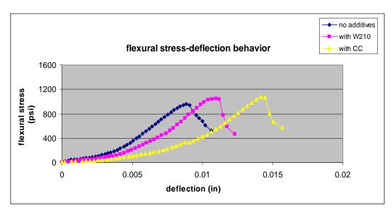
Figure 10. Influence of Alumino-Silicates on Modulus of Rupture: samples with gravel
