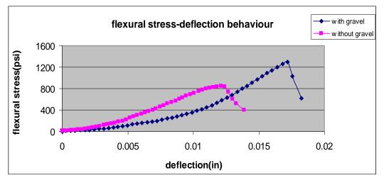
Figure 11. Influence of coarse aggregates on modulus of rupture
