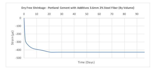
Figure 20. Shrinkage strain Vs Time: Portland cement with additives, 2% steel fibers
