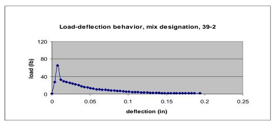
Figure 25. Load-deflection behavior of sample 39-2, fiber content of 0.5%
