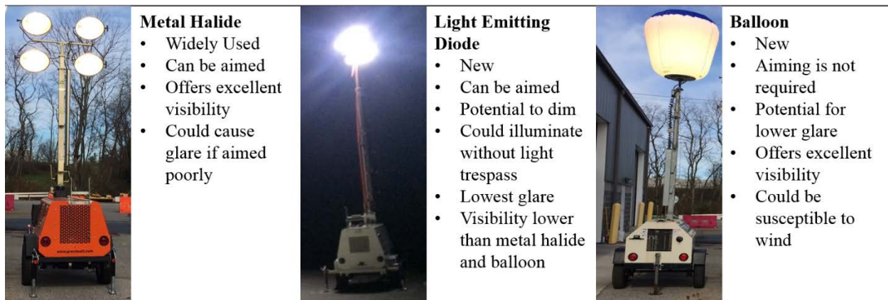
Figure 12. Features of the three light tower types used in the Virginia Smart Road evaluation.
