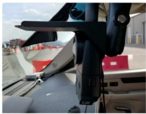
Figure 15. Mounting of the cosine-corrected illuminance meter on windshield to measure vertical illuminance levels.
