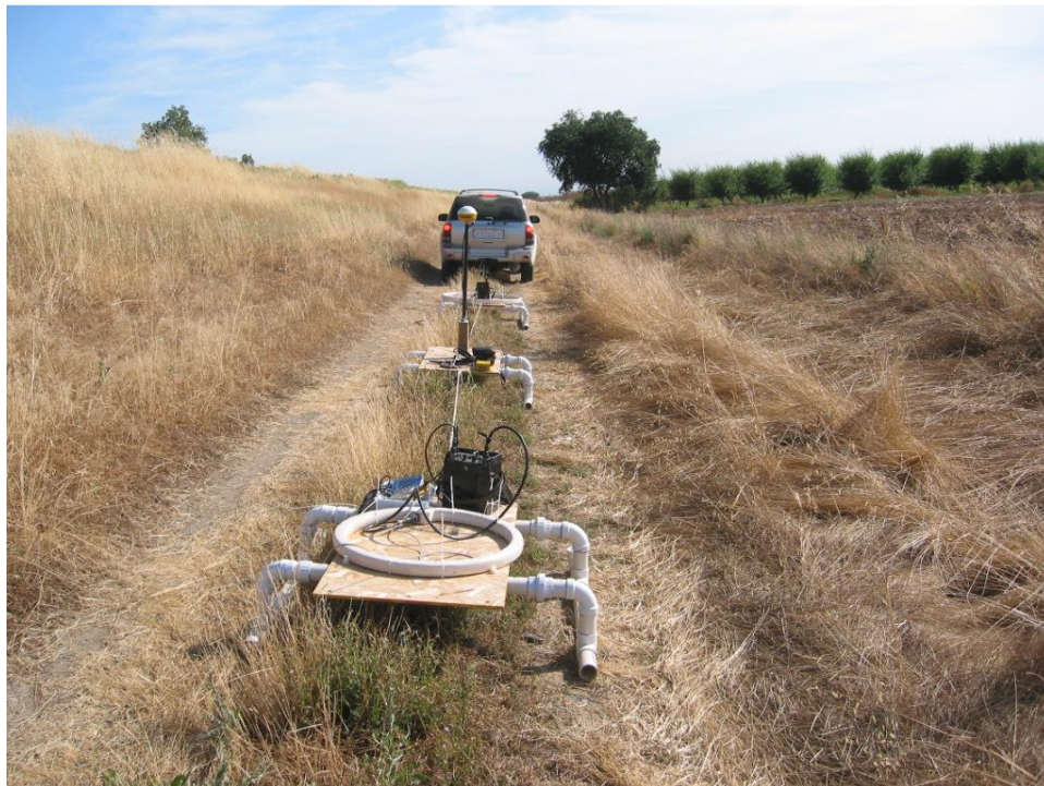
Figure 2-11 - Geonics Ltd. EM34 EM induction instrument being towed by a vehicle collecting continuous data (Llopis and Simms, 2007)
