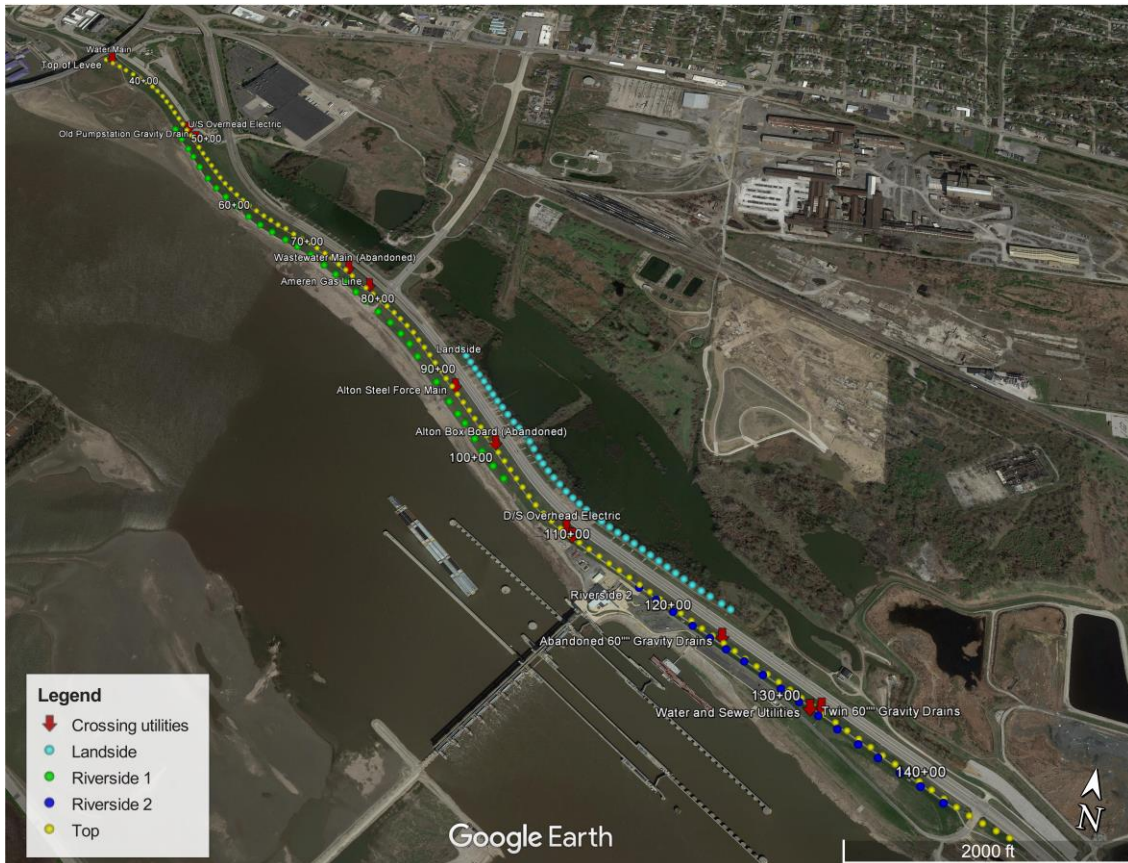
Figure 3-10. Survey paths for MASW and CCR at Mel Price Reach of the Wood River Levee
