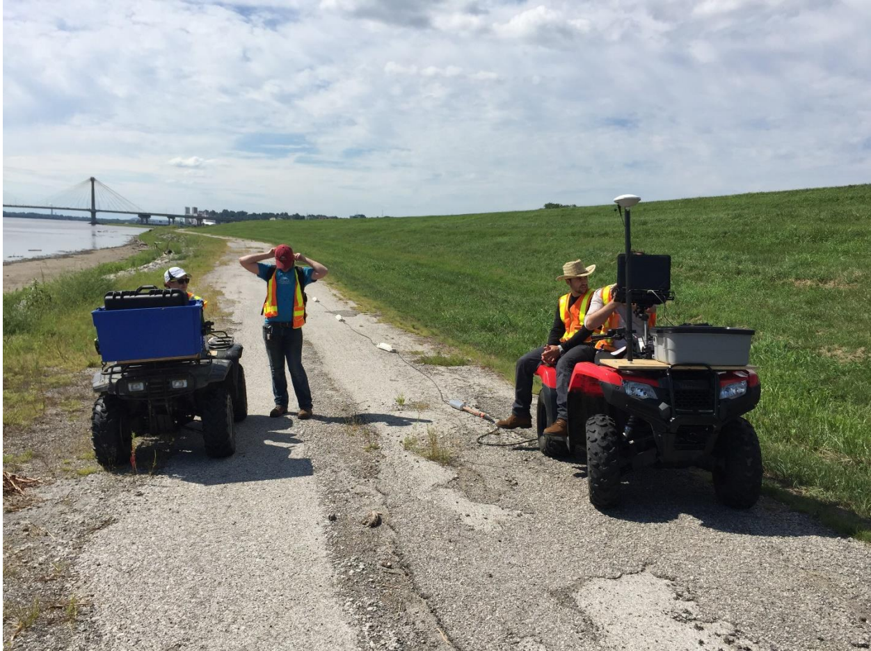
Figure 2-23 - CCR used to measure electrical resistivity at the toe of a levee close to the Mel Price Lock and Dam in Edwardsville, IL
