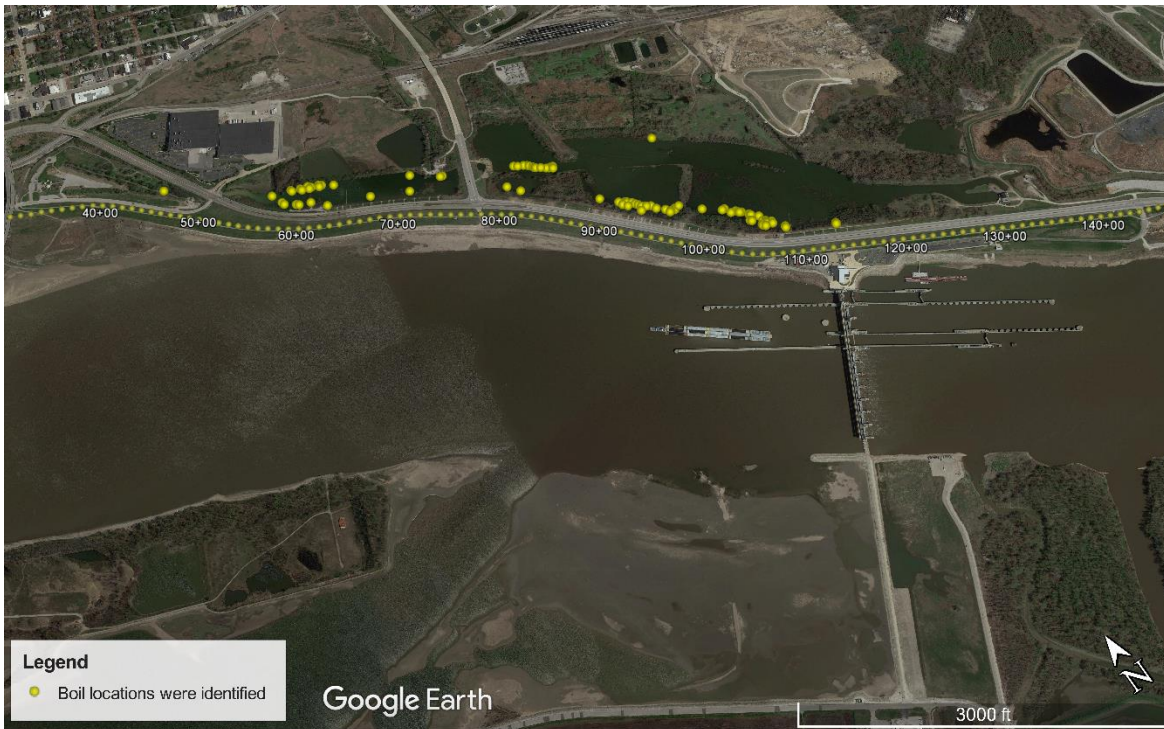
Figure 3-8. Melvin-Price Lock and Dam and Wood River Levee system. Levee centerline stationing and sand boil locations are shown (USACE, 2016).
