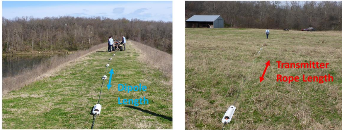
Figure 3-6. OhmMapper arrays: a) linear surveys pulled by ATV b) grid survey pulled by harness.
