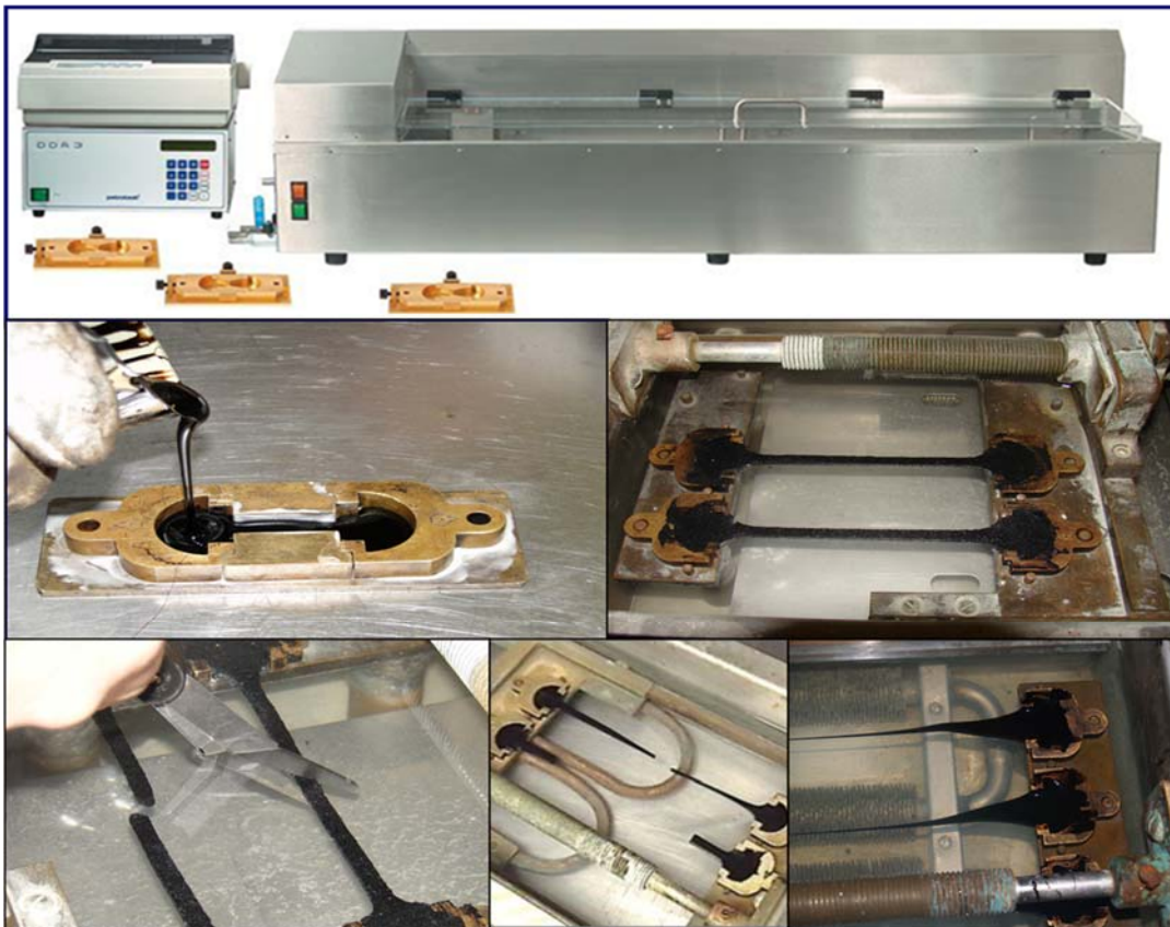
Figure 6 Typical ductilometer test setup
