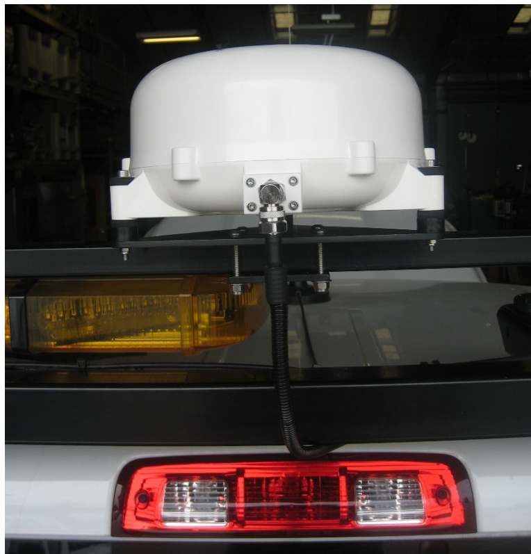
Figure 5.26: Satellite antenna mounted on vehicle light bar
