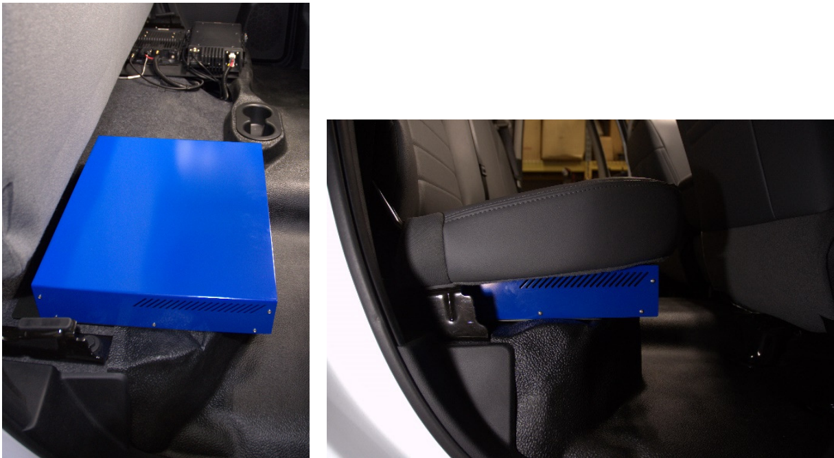
Figure 5.25: Responder system box mounted under right rear seat in vehicle
