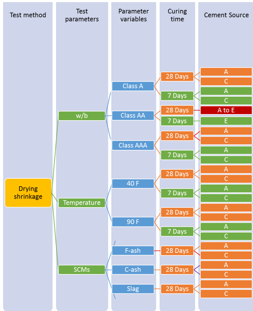
Figure 6.6: Experimental program for the drying shrinkage of concrete
