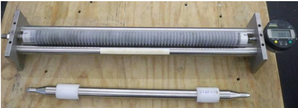
Figure 4.2: Autogenous shrinkage measured on a corrugated tube specimen, in accordance with ASTM C1698 [66].
