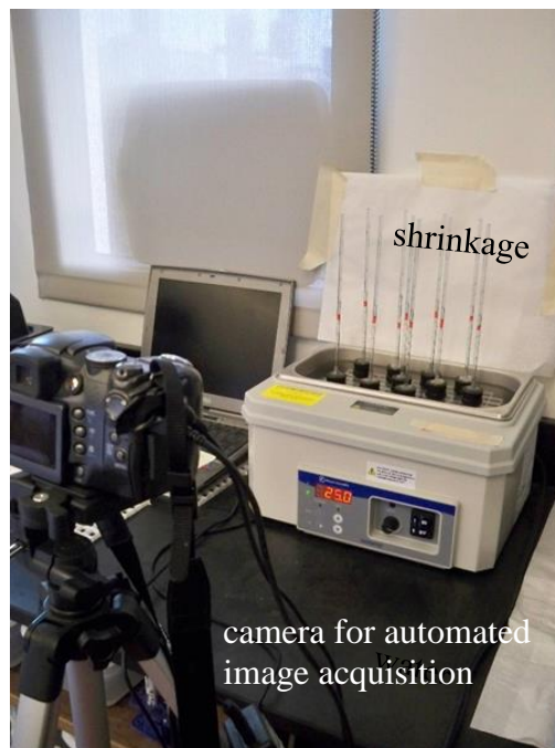
Figure 4.1. Experimental set-up used for chemical shrinkage test. Shrinkage was monitored by tracking the heights of red oil droplets atop the water within the capillary pipettes. Image acquisition software was used to automatically record images at 30 min intervals.
