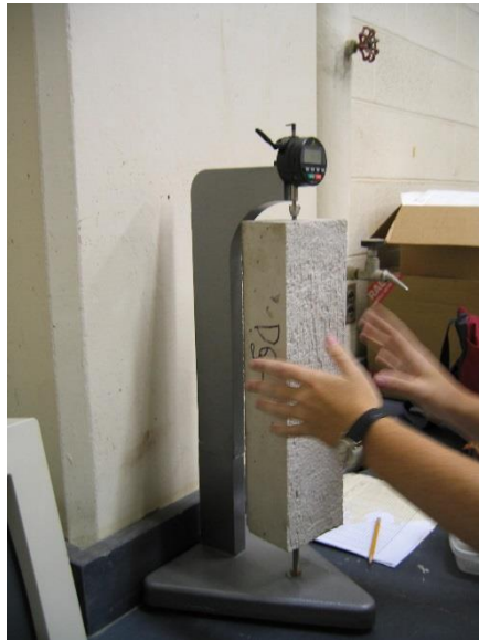
Figure 6.5: Drying shrinkage sample with length comparator
