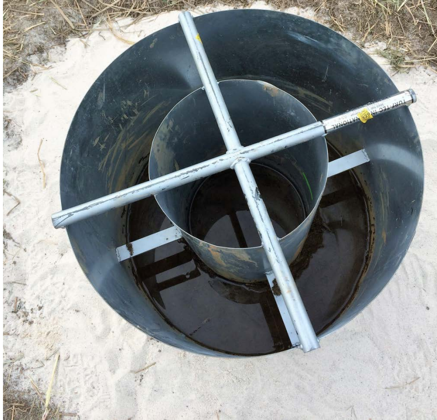
Figure 9. Falling-head DRI test in coarse filter sand in Canton, Georgia.
