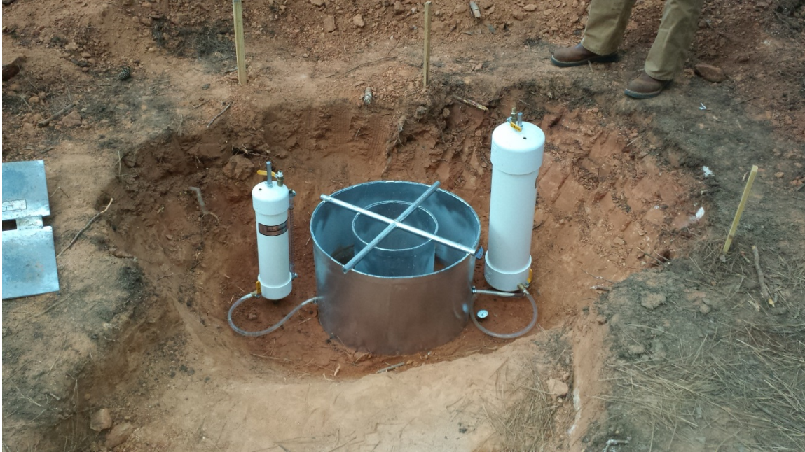
Figure 6. Test set up for in situ measurement of saturated hydraulic conductivity using a double-ring infiltrometer.
