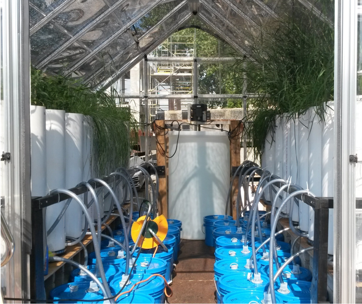
Figure 4: View of the greenhouse on sampling day with all columns, blue sample buckets, batch mixing can, and shade tarp.
