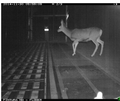
Figure 16. Mule Deer Doe Stood on I-15, Pintura Electric Pavement and Then Jumped Single Cattle Guard.
