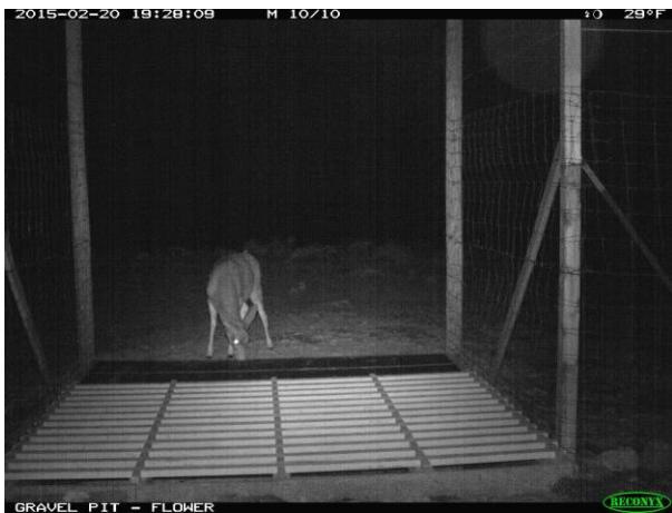
Figure 6. Mule Deer Doe is Repelled from Electric Pavement at Hardware Ranch, UT.
