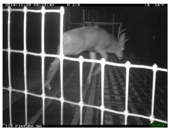
Figure 15. Mule Deer Buck Walked onto I-15 Pintura Electric Pavement, Then Leaped and Moved Across Single Cattle Guard.
