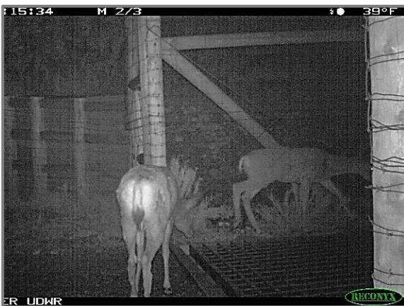
Figure 26. Mule Deer Walked Along Edge of Wildlife Guard on US 91, Left, and Walked Across Top of Electric Mats near US 6, Right.
