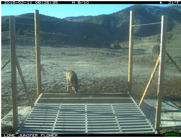
Figure 5. Mule Deer Fawn is Repelled from Electric Pavement at Hardware Ranch, UT.
