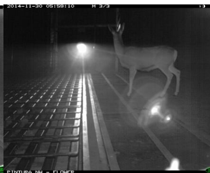
Figure 16. Mule Deer Doe Stood on I-15, Pintura Electric Pavement and Then Jumped Single Cattle Guard.
