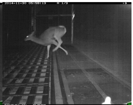
Figure 16. Mule Deer Doe Stood on I-15, Pintura Electric Pavement and Then Jumped Single Cattle Guard.
