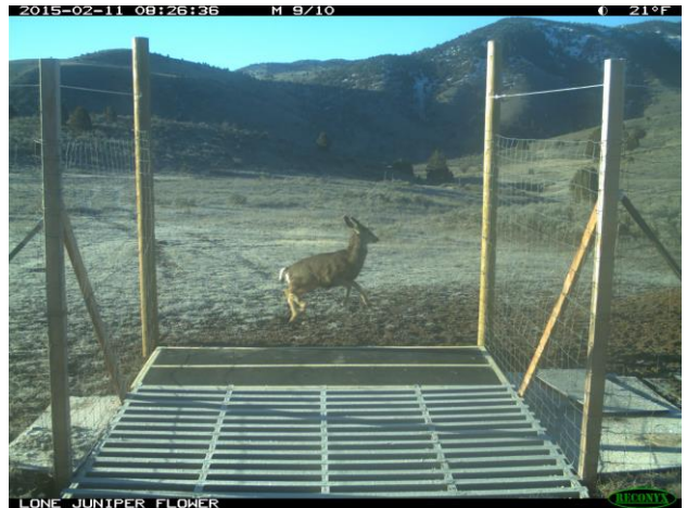
Figure 5. Mule Deer Fawn is Repelled from Electric Pavement at Hardware Ranch, UT.
