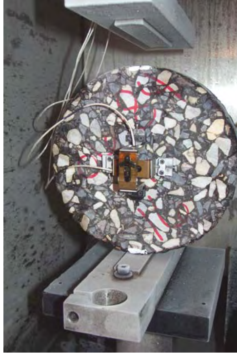
Figure 2: Instrumented IDT Specimen
