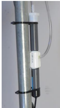
Figure 13: Conductivity sensor (black bottom endcap) and ion exchange filter (upper tube with white endcap).
