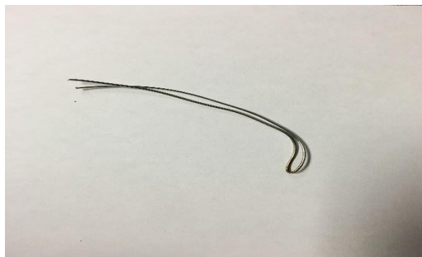
Figure 8: Stainless steel wire loop tool for loosening coil specimen from bolt.
