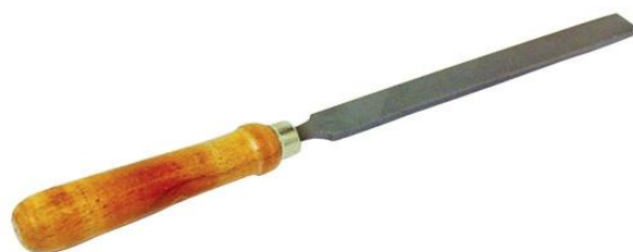
Figure 7: Hand file used to remove corrosion products from plates.
