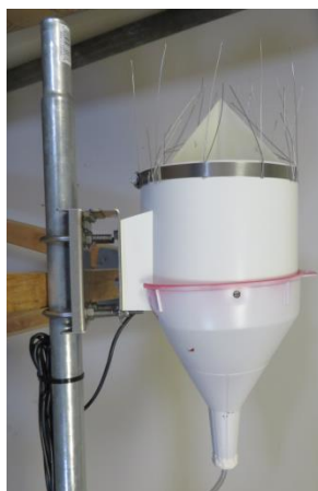
Figure 11: Rain gauge – bird deterrence and particle baffle.
