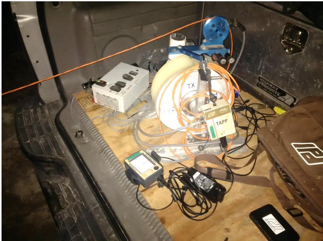
Figure 2.9 Automated reel and data collection system used for probe testing.
