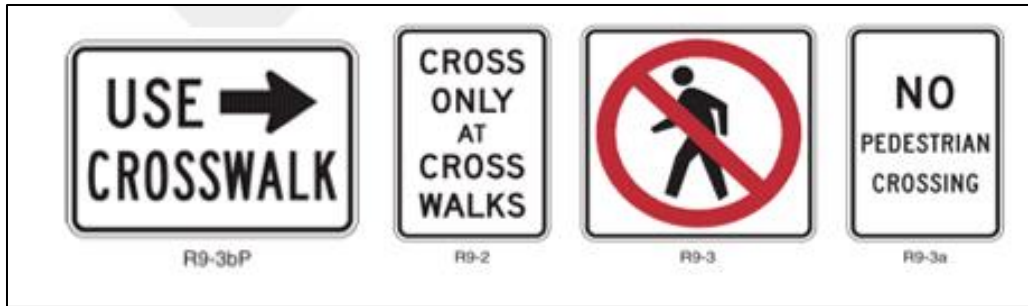
Figure 62. Pedestrian signs used in conjunction with fencing.
