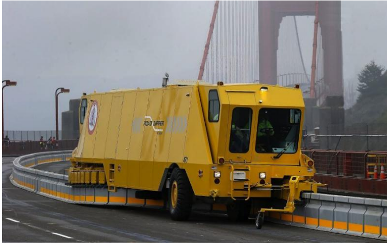
Figure 2-12 MTBS working within work zone (Lindsay, 2015)
