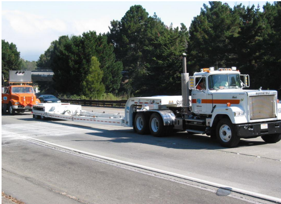
Figure 4-4 Using Balsi Beam mobile work zone barrier in the field (Caltrans, 2004)
