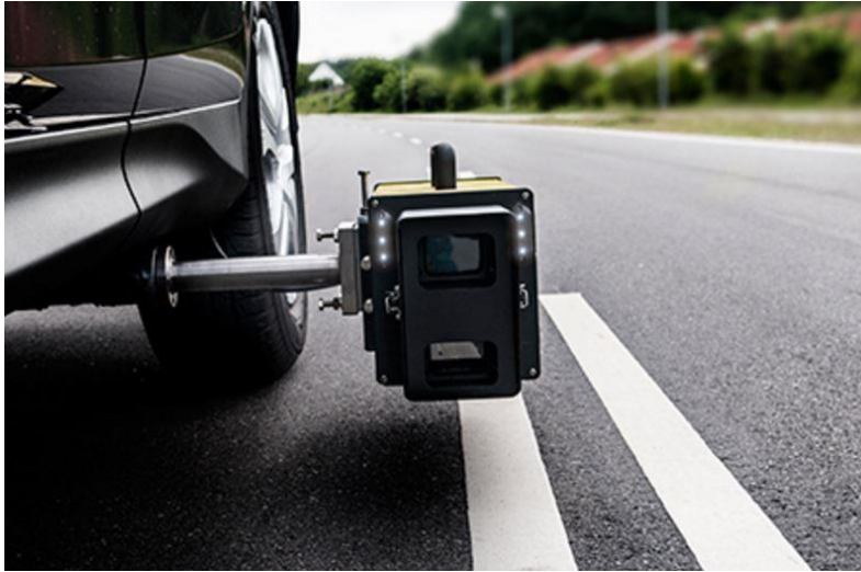
Figure 2-1 LTL-M, a mobile retroreflectometer unit by Delta (Delta, 2016)
