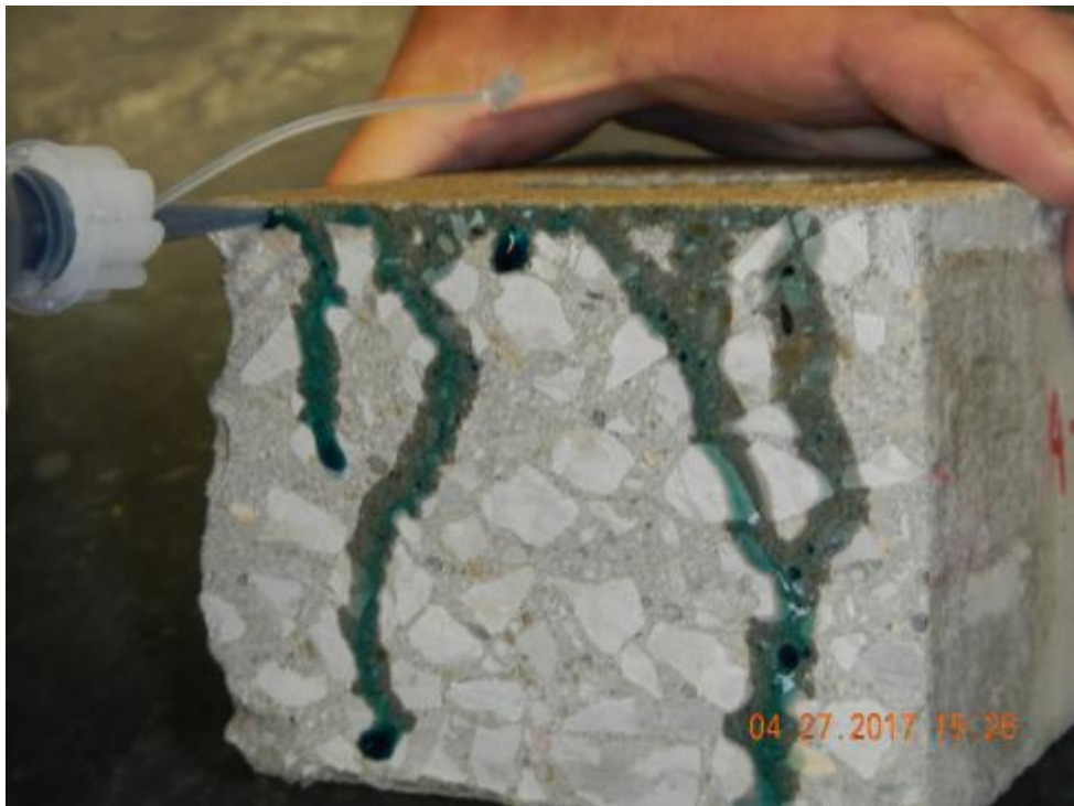
Figure 16 Dye Application for Depth of Penetration Testing
