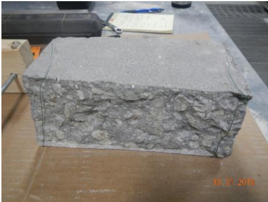
Figure 3 Fractured Surface with Wire Spacer
