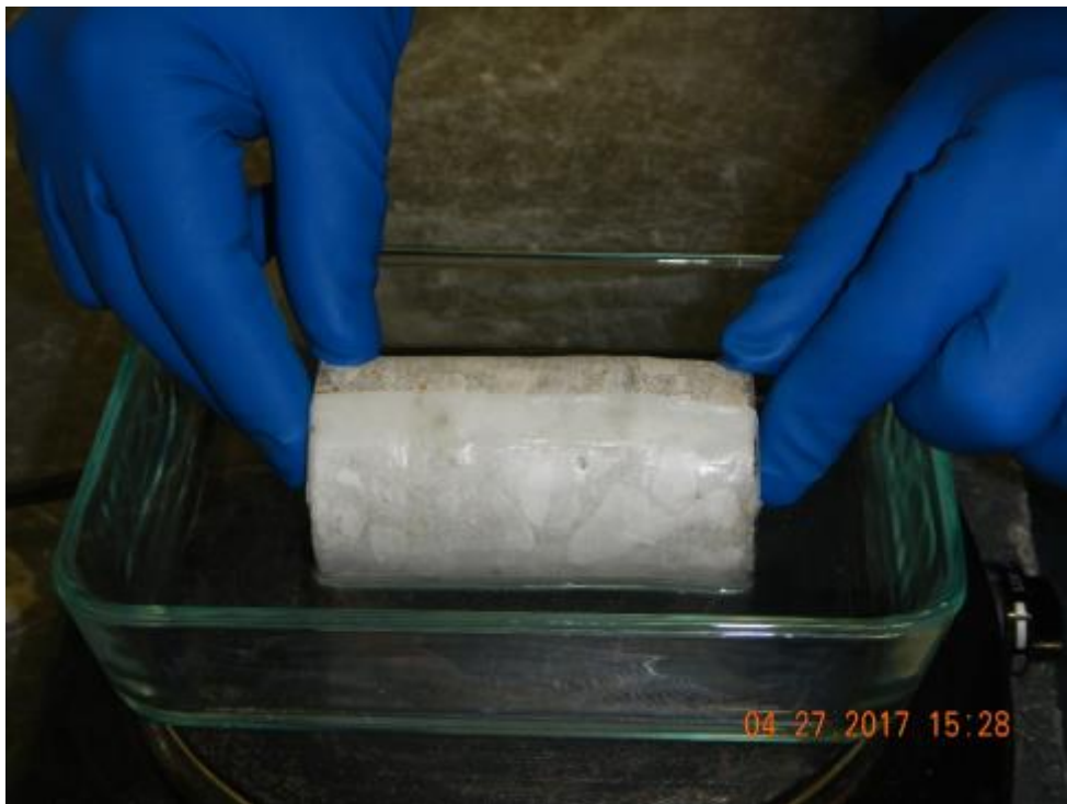
Figure 14 Application of Paraffin with Ends Taped
