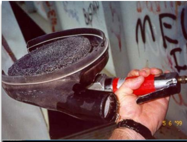
Figure 21. A Power Tool (Grinder) with Non-Woven Abrasive Pad and Vacuum Shroud
