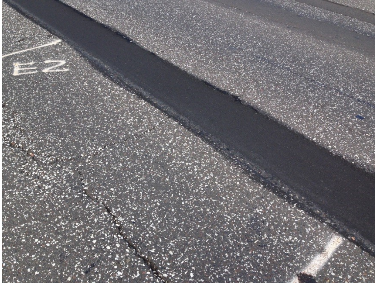
Figure 3.78 Pothole E-2 (28 Days after Patching).
