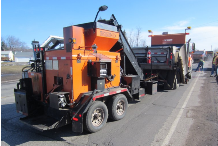
Figure 2.1 Stepp SRM 10-120 Asphalt Recycler.
