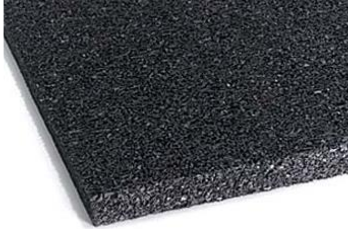
Figure 23. Recycled Rubber Used in Noise Wall Applications.
