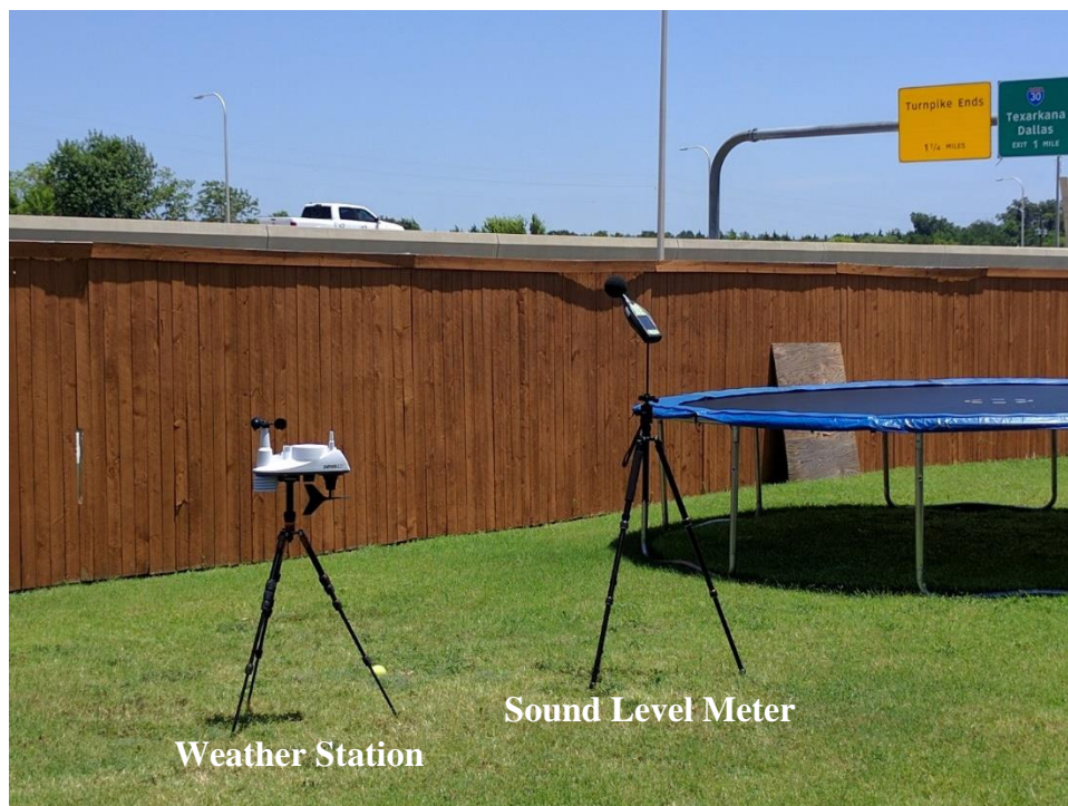
Figure 11. View of Sound Level Meter and Weather Station Setup at Monitoring Location with Line of Sight to Highway.
