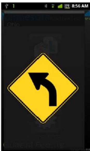
Figure 4: Example of MRFT In-vehicle Signage Warning (Curve Warning)
