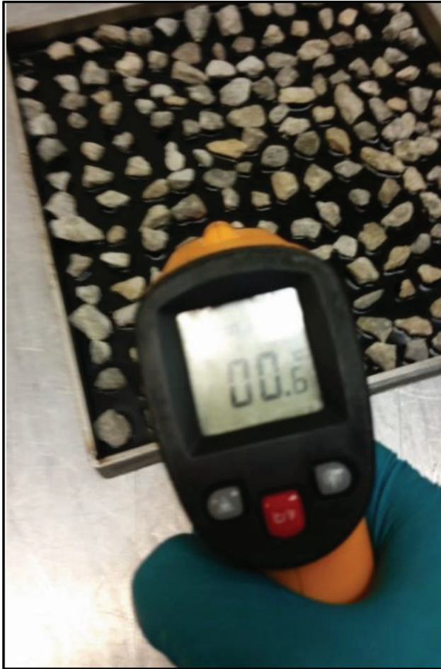
Figure 3.19 Specimen temperature after freezer conditioning, 32 \pm 2 °F ( 0 \pm 1 °C).
