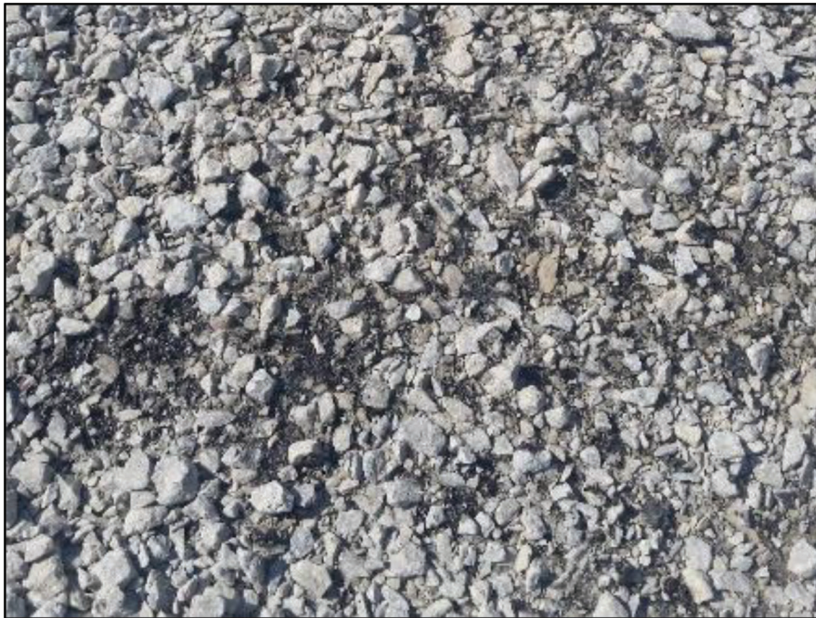
Figure 3.15 Aggregate loss at area subjected to broom's shear force.
