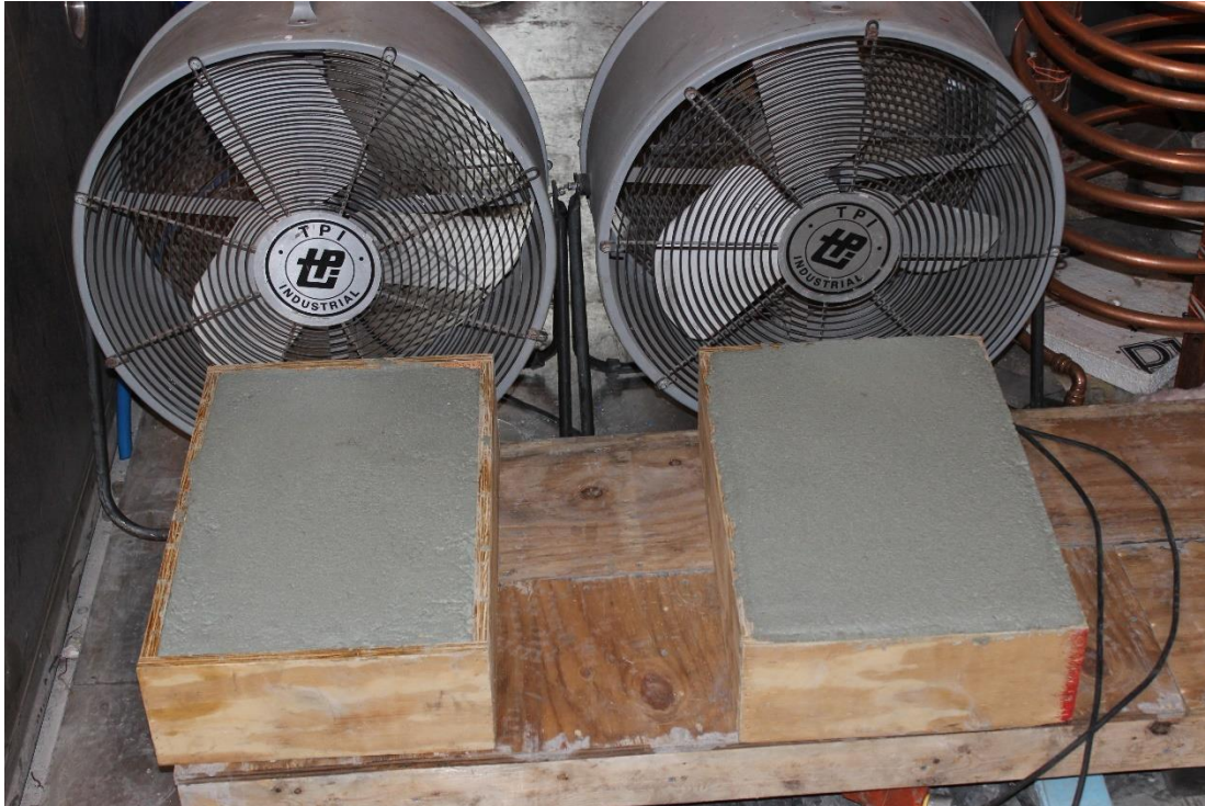
Figure 1: Experimental testing setup for plastic shrinkage
