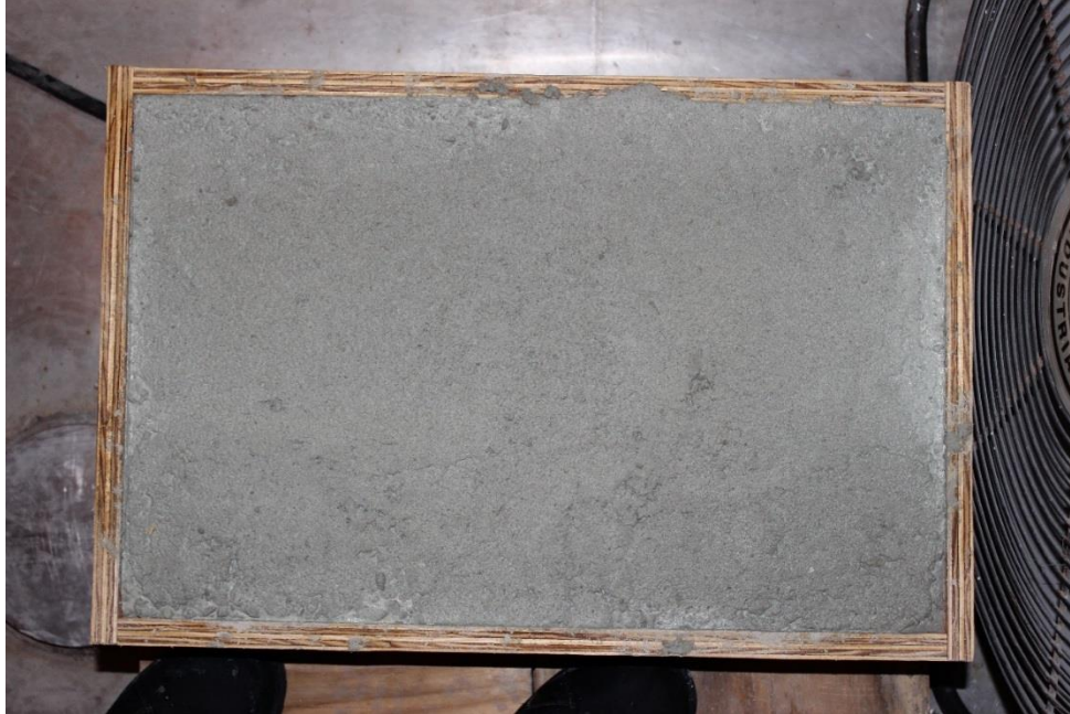
Figure 3: Plastic shrinkage specimen with fresh concrete
