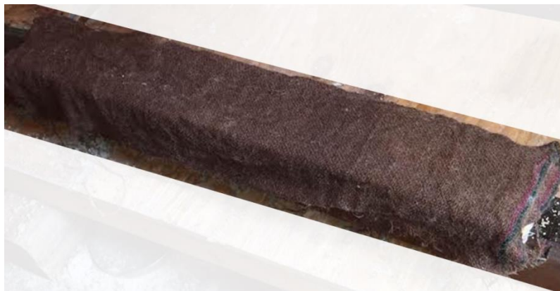
Figure 23: Photograph of curing condition (b): Curing with initially saturated burlap, no plastic sheet applied.
