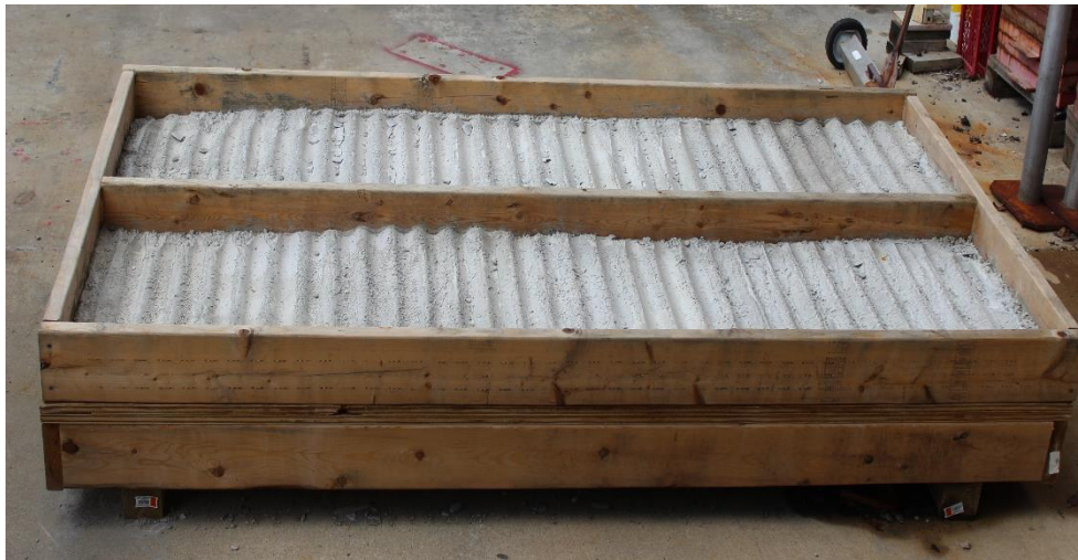
Figure 9: Corrugated concrete base layer simulating a surface-roughened pavement.
