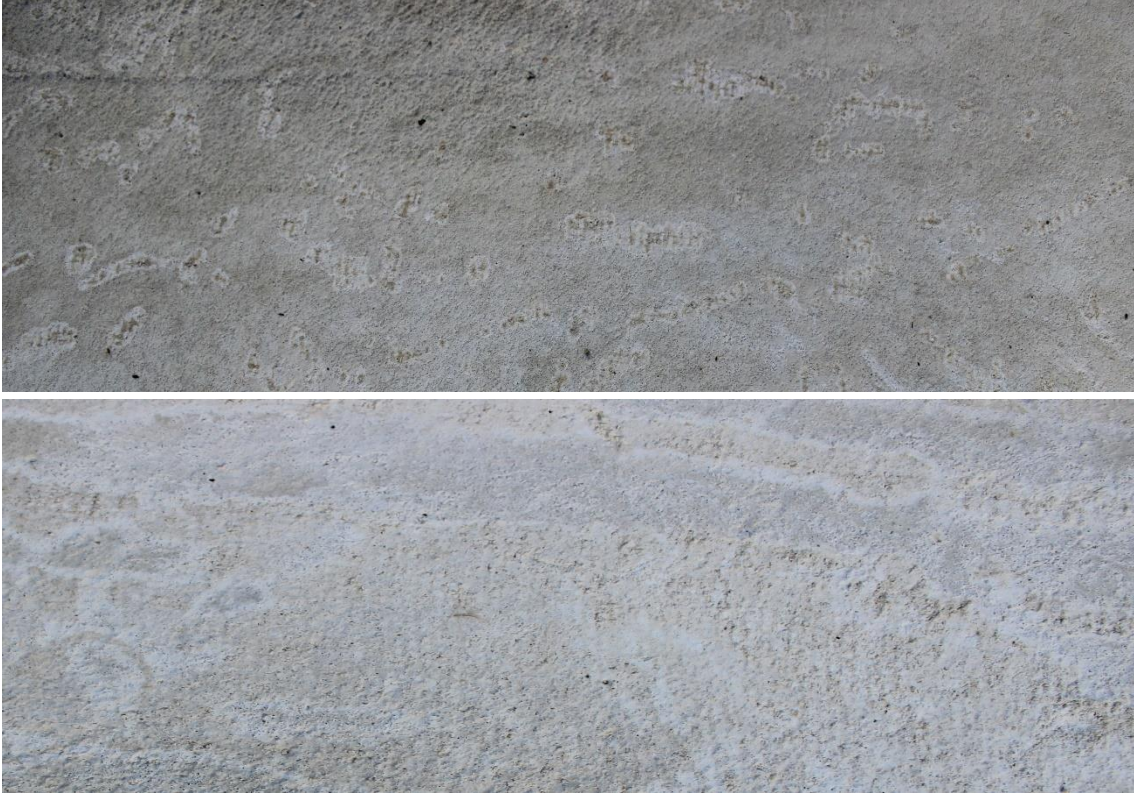
Figure 36: Photograph of LMC overlays after 21 days.
