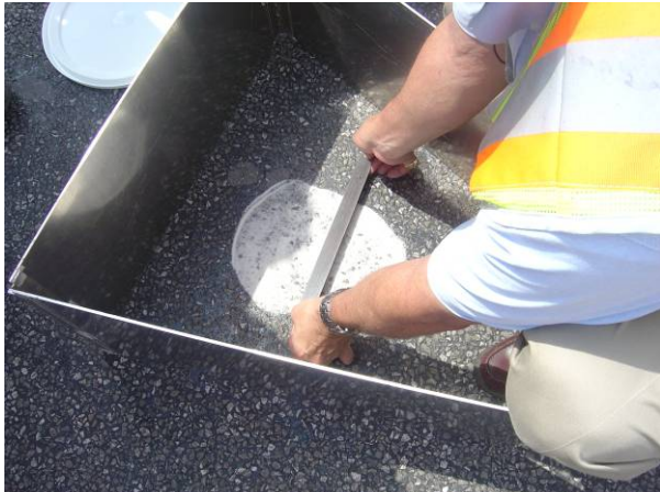
Figure 8. Measuring the Diameter of the Sand Patch
