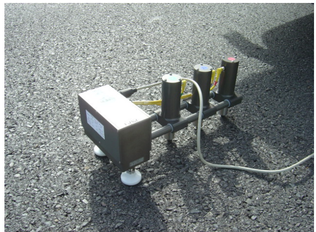
Portable Seismic Pavement Analyzer Equipment
