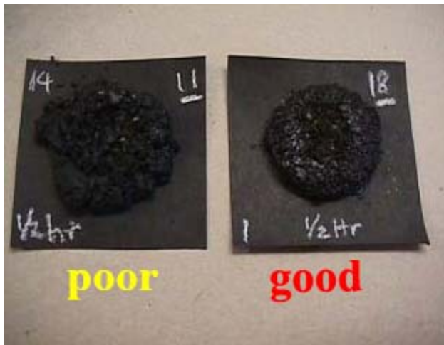
Cohesion Test Results
