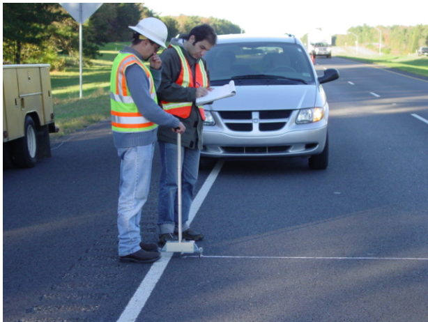
Rut depth measurement
