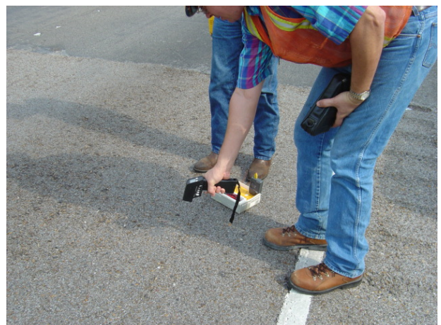
Temperature measurements for Falling Weight Deflectometer
