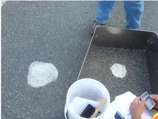
Figure 9. High Pavement Texture Difference
