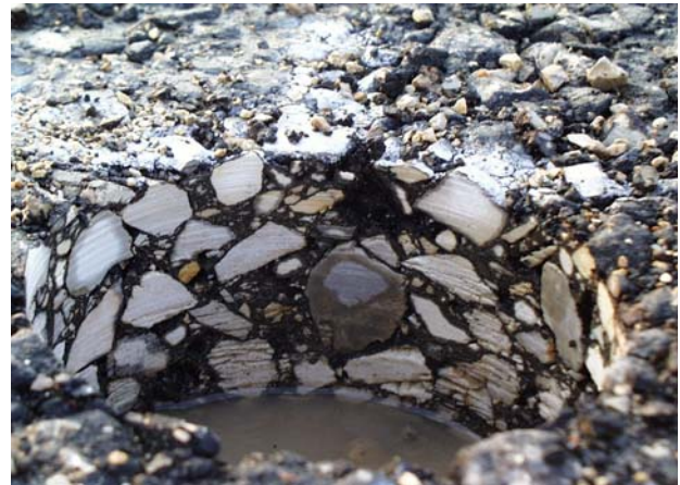
Aggregate breakdown during coring operation
