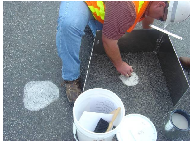
Figure 9. Performing the Sand Patch Test
