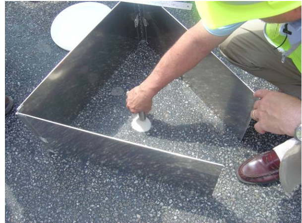
Figure 6. The Sand Patch Test
