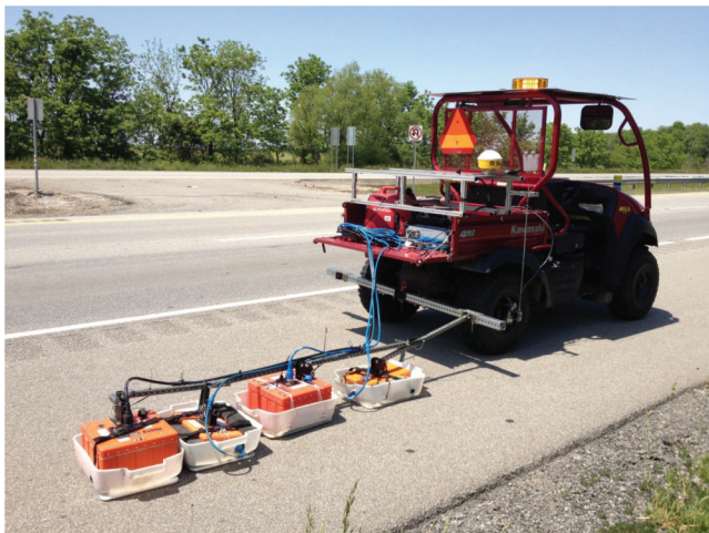
Figure 7.1 GPR Equipment set up on the side of I-65N.
