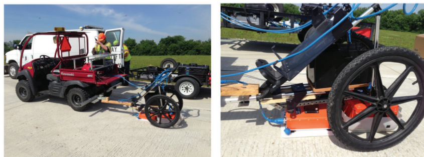
Figure 8.3 Field Setup of dual frequency system (900 MHz and 400 MHz).
