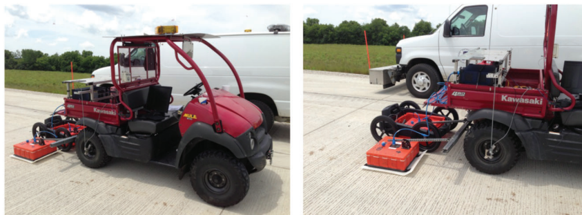
Figure 8.7 Field setup of dual-parallel configuration (270 MHz).
