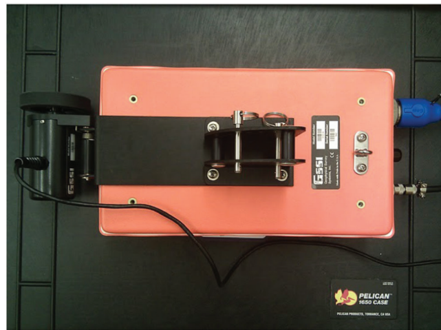
Figure 4.3 Model 3101 900 MHz antenna attached to a Model 611 survey wheel.
