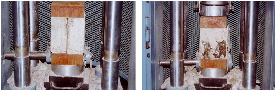
**Figure 4: Uniaxial test with (a) a damaged concrete cube, (b) a concrete cube repaired with epoxy resin (Issa and Debs, 2007)**
