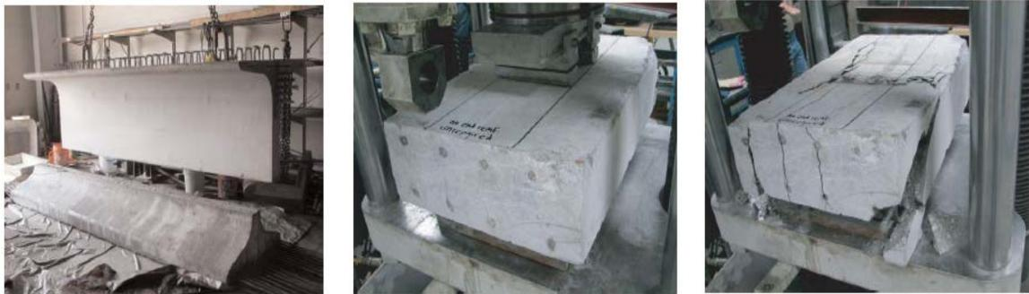
**a. Bottom flange completely cut from the specimen.**
