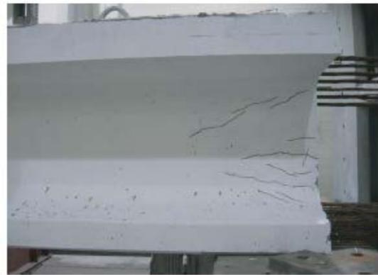
**Figure 2: Longitudinal cracks due to pre-stress transfer in a 42-ft long, 45-in high Bulb-T girder (Tadros et al., 2010)**
