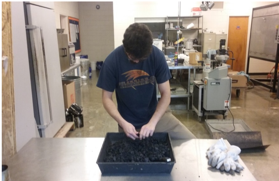
Figure 2-11 Separating aggregate in asphalt mixtures
