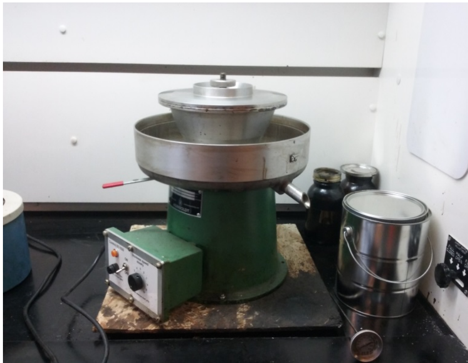
Figure 2-4 Centrifuge for RAP extraction
