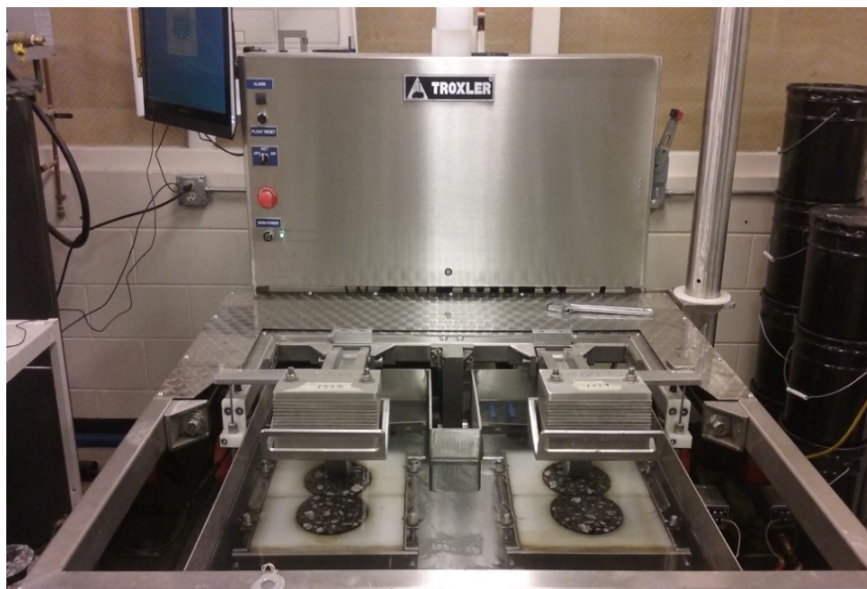
Figure 2-14 Hamburg Wheel-Tracking Device
