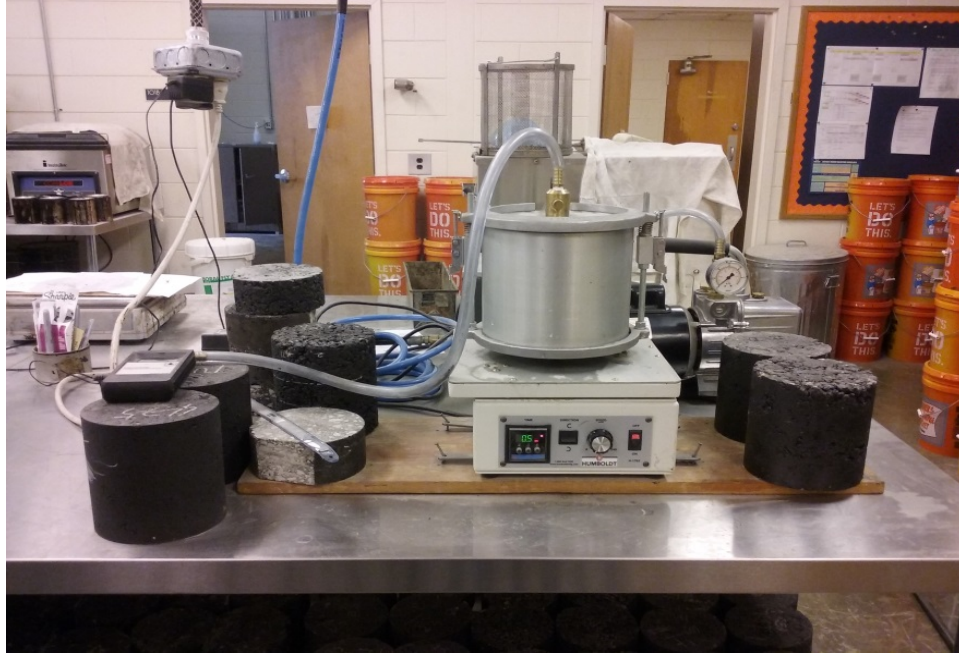
Figure 2-12 Apparatus for Measuring Theoretical Maximum Density
