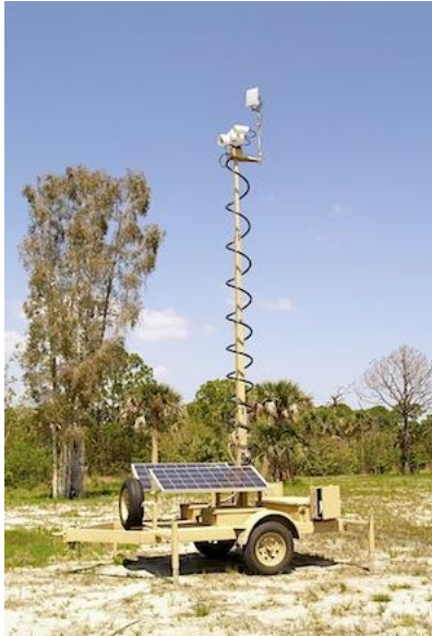
Figure 5 - EMX International Mobile Surveillance Trailer
