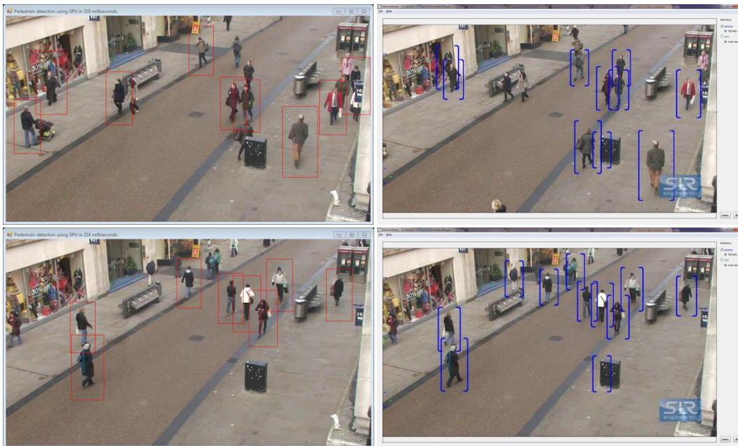
Figure 6 - Pedestrian Detection Output for OpenCV (left) and SLR Engineering (right)
