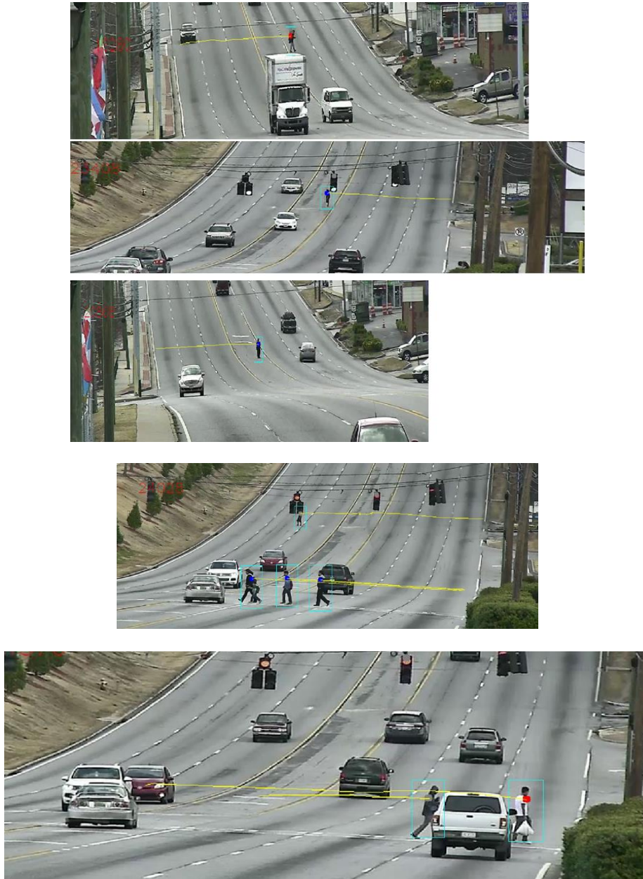
Figure 27 - Sample Pedestrian Detector Output
