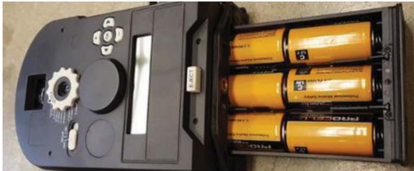
(e) Time-lapse camera takes C-cell batteries
