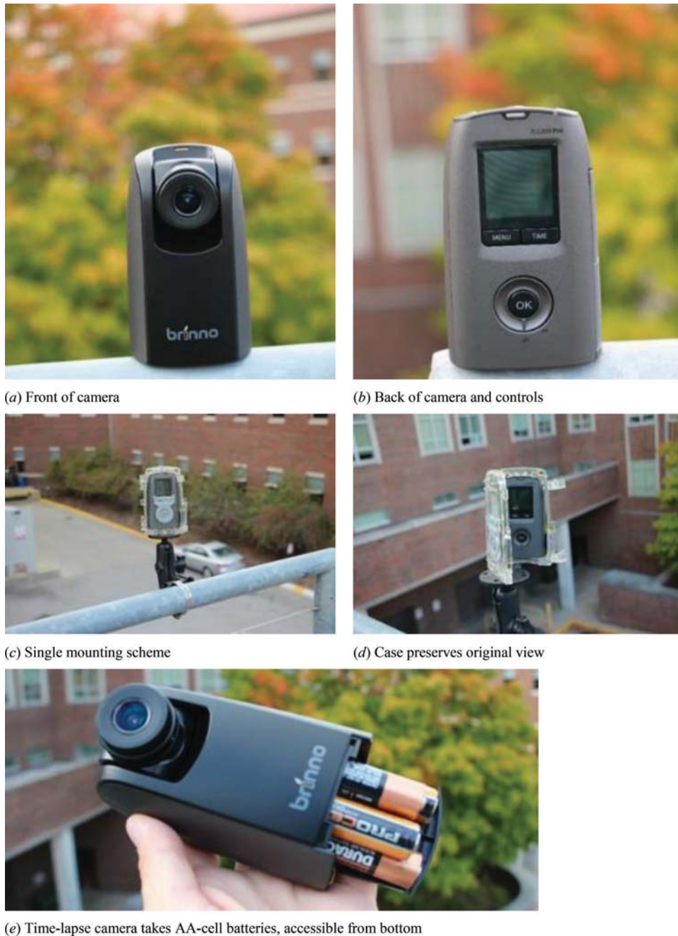
Figure 1.3 Brinno time-lapse camera details.
