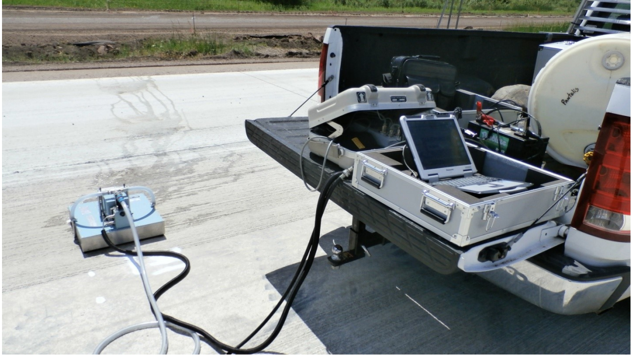
Figure 2-5 Dynamic Friction Tester (ASTM E 1911) used for friction evaluation in this project
