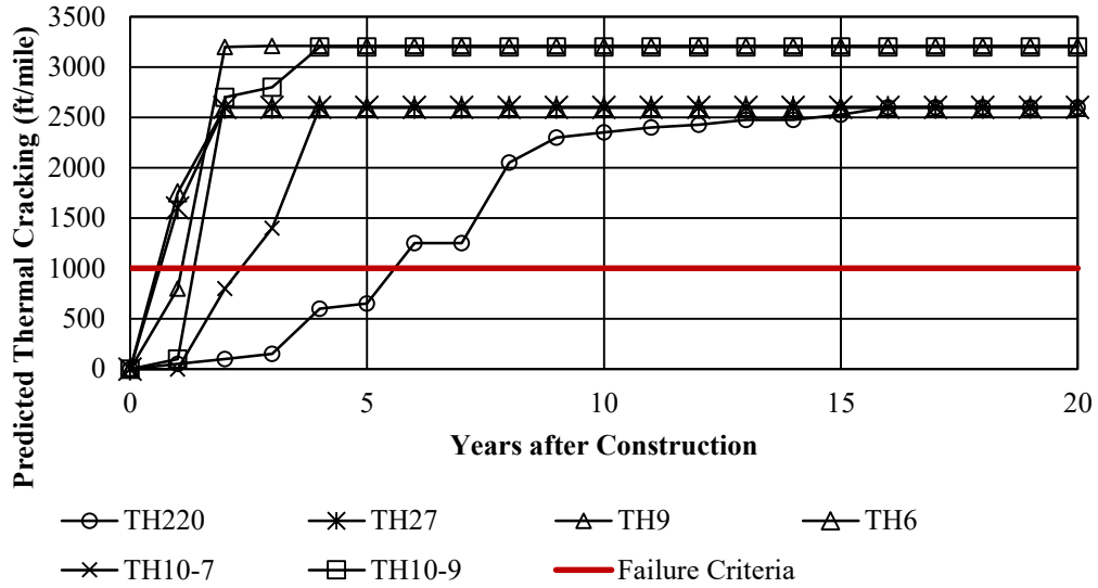
Figure 7.2: Pavement ME Predicted Thermal Cracking for Field Sections.
