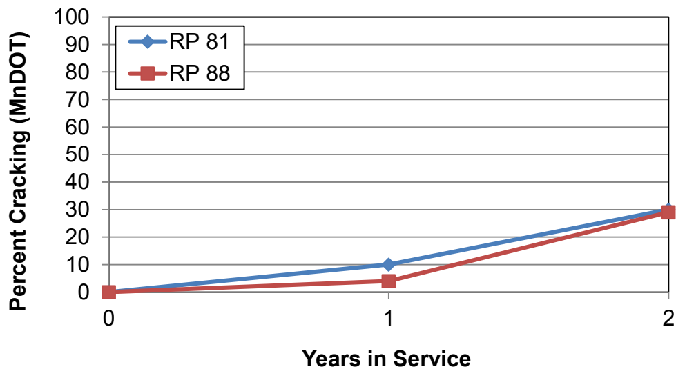
Figure 6.8: Cracking performance of TH 28 (SP 6104-11)
