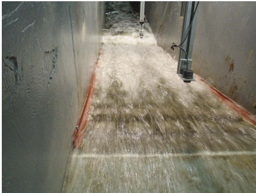
Figure 4.92. View looking downstream from the shoulder during 1 to 1.5 hour run with flow of 2 \text{ ft}^3/\text{s} and overtopping depth of 3 inches. The flow was aerated and very turbulent.
