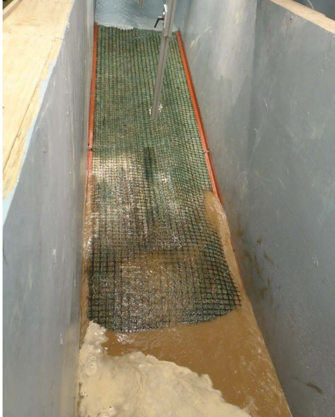
Figure 4.22. Post flow erosion after 2.7cfs testing. Note the mound near bottom of slope and depression along the left side of the flume looking upstream. Sediment rich water on slope and in tail water indicating erosion occurring on the slope under the ECB.
