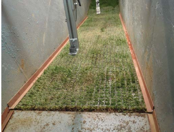
Figure 4.54. Looking downstream from shoulder. Installed sod and geogrid before testing.
