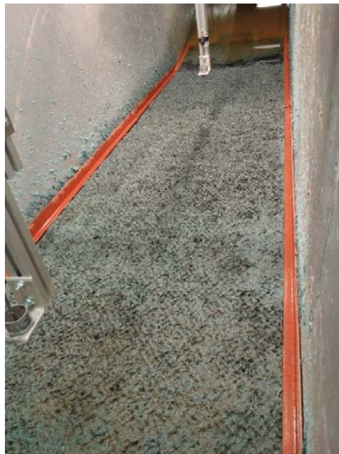
Figure 4.73. View from upstream after 1 hour of run time, note that some of the FRM has been washed away from the surface of the TRM.
