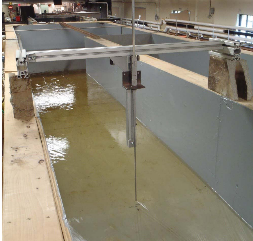
Figure 3.21. Point gauge at road crest in use to measure depth of flow over the crest of the model road cross section.
