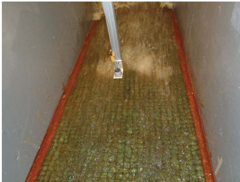
Figure 4.21. Start of erosion about \frac{1}{2} way down the slope indicated by the depression leading to a mound that aerated the flow in the center of the flume. Looking downslope from shoulder at mound and hydraulic jump.
