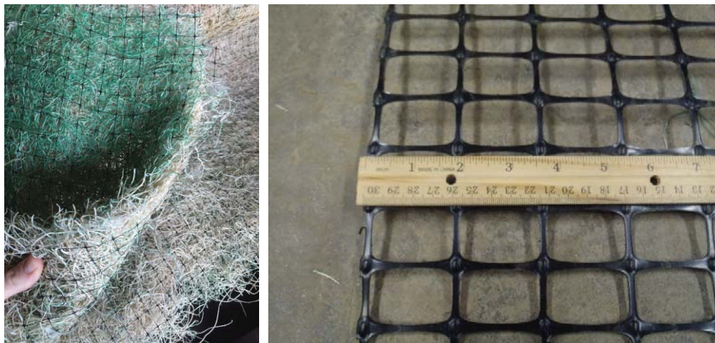
Figure 3.10. Layers of the armored sod. Image on the left shows the layers of the Erosion Control Blanket. Image on the right shows the plastic geogrid.
