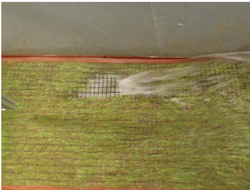
Figure 4.64. Aerial view of the slope just past halfway down the slope a large depression formed quickly at the seam of two pieces of sod just minutes before the end of the 2-4 hours testing time.
