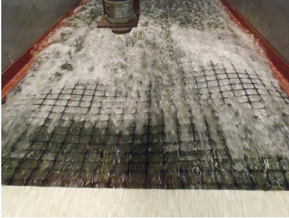
Figure 4.46. Looking downstream from the shoulder during 2-4 hour testing period. Note the large area of erosion occurring near the shoulder specifically near the left wall.
