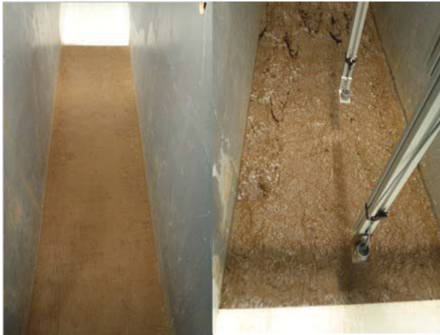
Figure 4.14. (Left). Looking upstream at 4H:1V slope with extended pavement (white) before testing. (Right). Looking downstream at flow over 4H:1V slope during 2-4 minute run no prevalent channel on upper slope. Channelization begins on the lower portion of slope.
