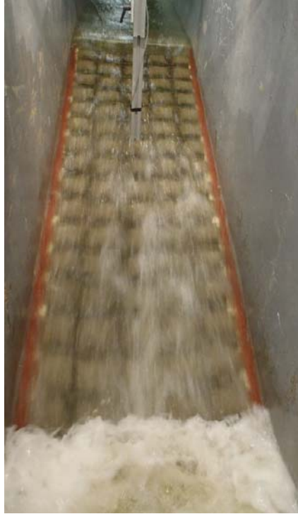
Figure 4.93. Looking upstream at slope near end of 1.5 hour run. Aeration near mid-slope and erosion/deposition areas stepping down the slope.
