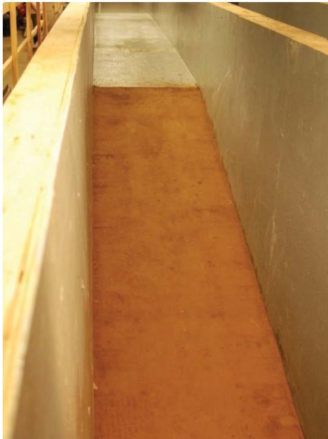
Figure 3.6. Prepared bare soil slope in the flume.
