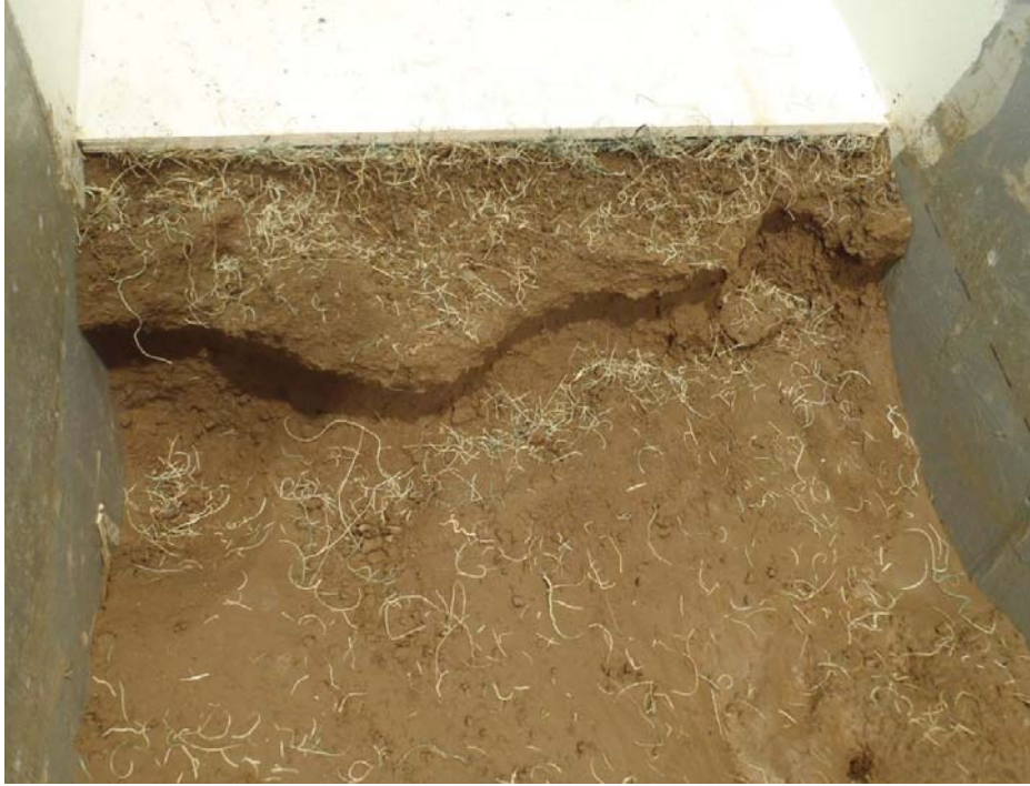
Figure 4.48. Looking upstream at shoulder and slope after stabilization material was removed. Note the remaining soil that was not undermined but close to it after 6 hours of run time.
