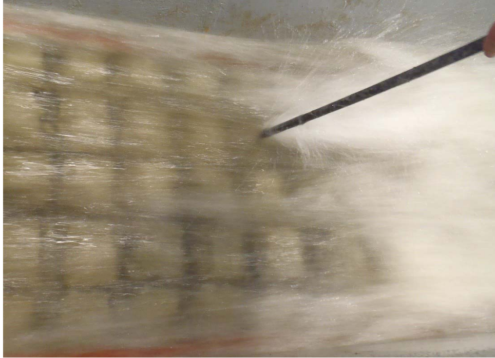
Figure 6.2. Flexible concrete geogrid mat tested on the 4H:1V slope at 9.90 ft 3 /s and approximately 25 hours of run time. Concrete blocks may be pushed down with a probe rod 3-4 inches before touching the slope surface \frac{3}{4} of the way down the slope.
