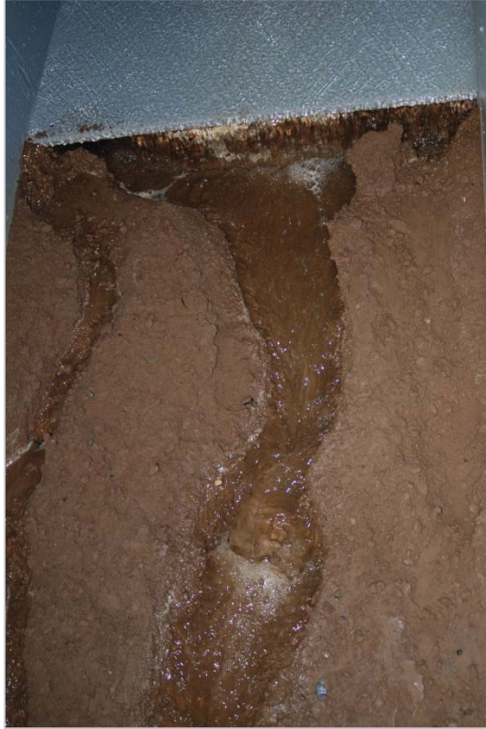
Figure 4.9. Channelized flow and separation from the edge of the shoulder forming trough at the transition.
