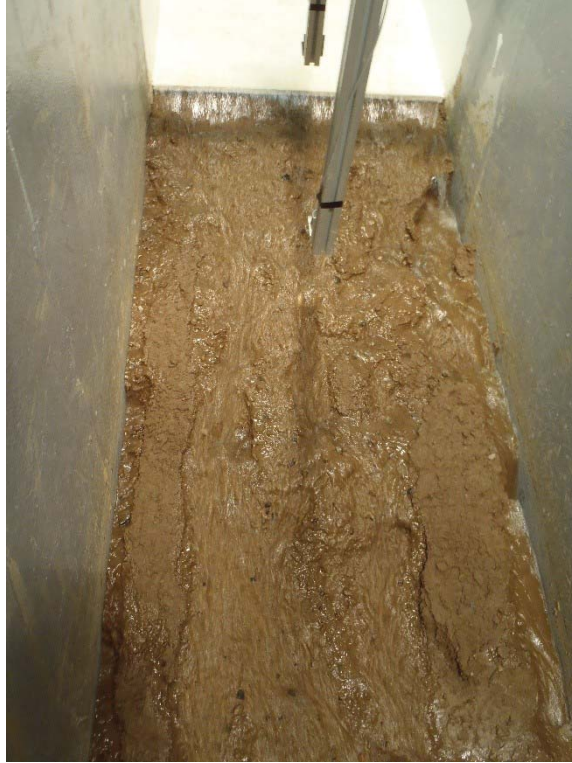
Figure 4.15. Looking upstream after approximately 25 minutes of run time. Channels and depressions forming, no trough or main channel forming.
