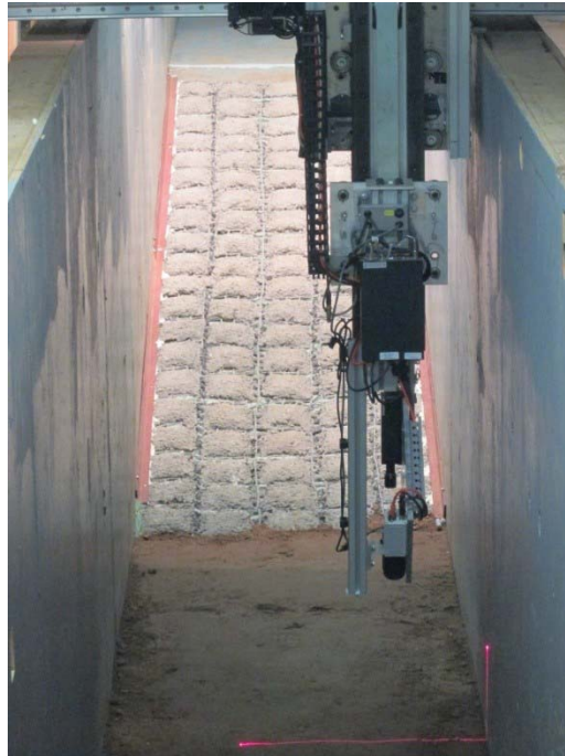
Figure 3.5. SAFL data acquisition carriage scanning pre-flow topography. The laser sheet is projected onto the soil near the bottom of the photo.
