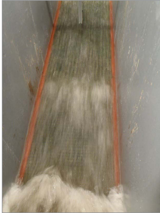
Figure 4.31. Flow on slope becoming aerated because of the increasing depth of erosion and separation of the geogrid from the soil. The image shows the formation of a hydraulic jump at bottom of the slope.
