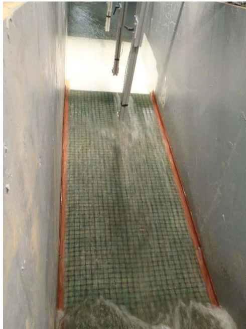
Figure 4.45. Looking upstream after 1.5 hours of run time. Erosion is observed 1.5ft downstream from the shoulder in the river-left half of flume.
