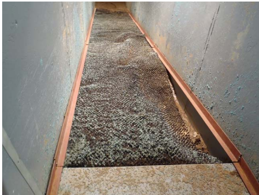
Figure 4.85. View looking downstream after 8.25 hours of run time. The large amount of erosion along right wall represents failure.
