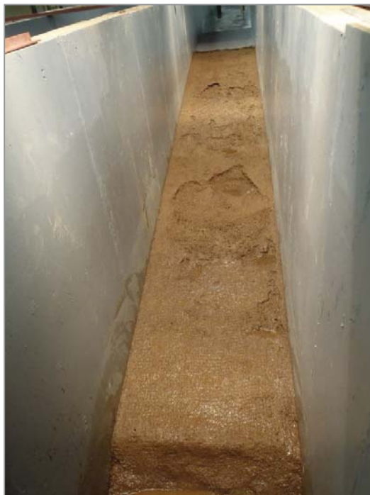
Figure 4.32. Looking upstream at bare soil post run with treatment removed showing different locations of erosion on the slope.
