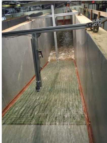
Figure 4.37. Looking downstream at slope with indications of immediate erosion by murky tail-water during the first test.
