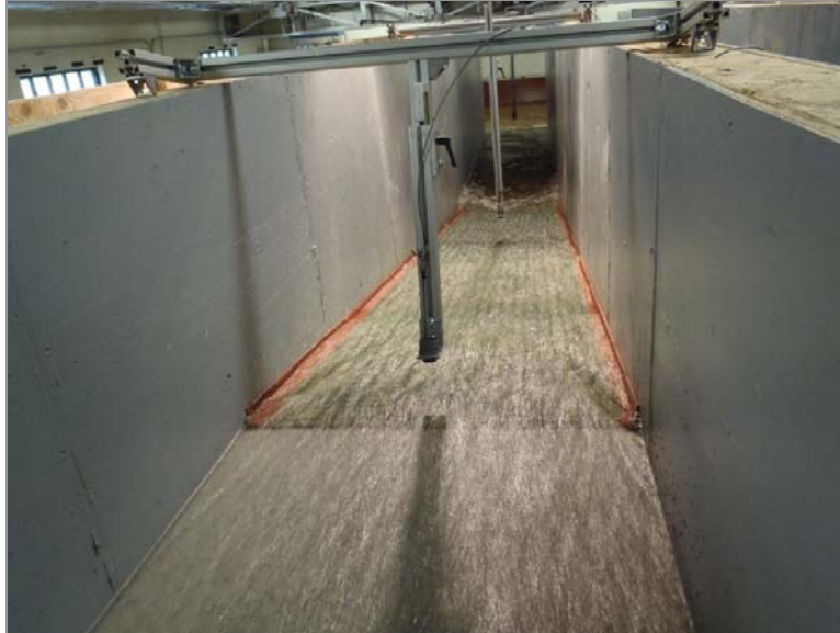
Figure 4.29. Running at 1cfs on 6H:1V slope. View from shoulder looking downstream in flume.
