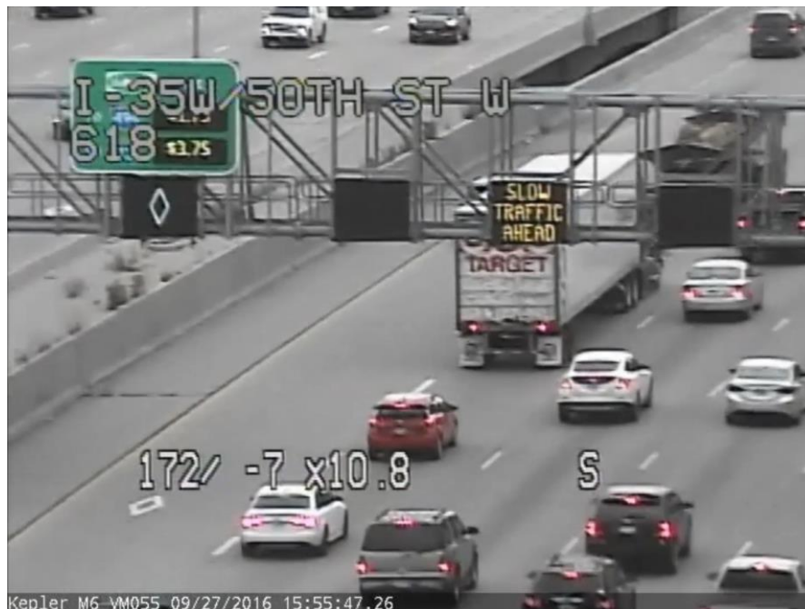
Figure 3.11 The queue warning system displaying warning message
