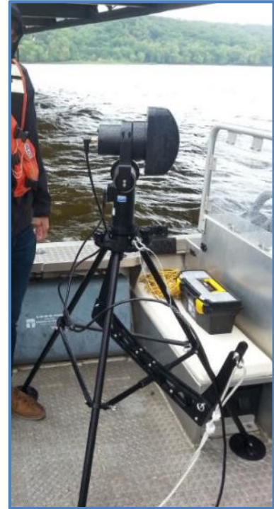
Figure 7.1 – MnDOT’s Teledyne Blueview BV1350 Sonar Scanner
