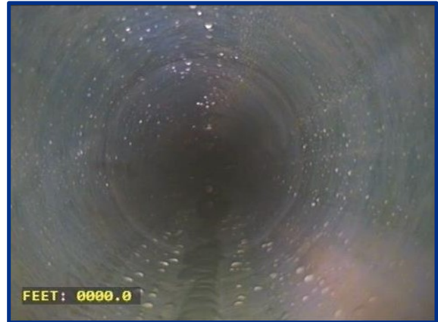
Figure 5.4 – Footage Counter on a CCTV Camera Screen
