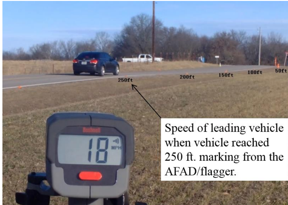
Figure 2.3.4 MOE 1 example: Speed of the Leading Vehicle at 250 ft. from the AFAD/Flagger
