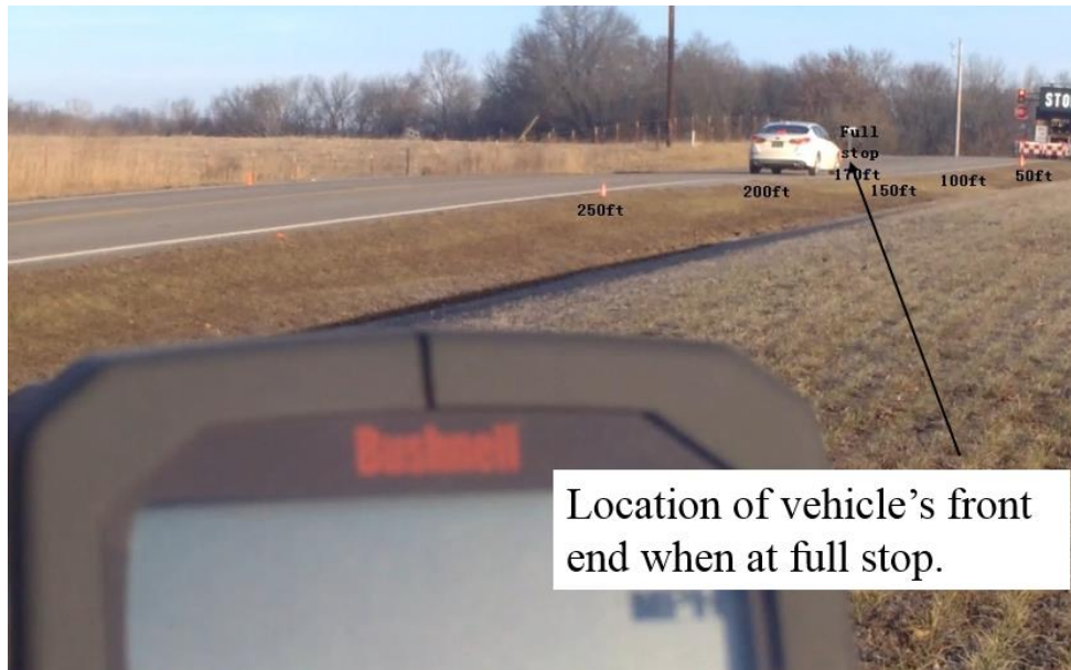
Figure 2.3.5 MOE 2 example: Full Stop Location
