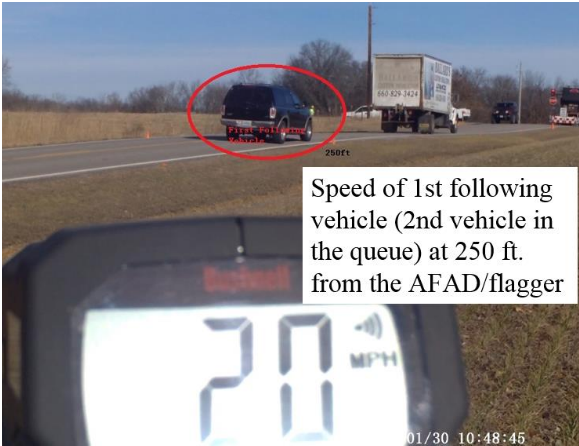
Figure 2.3.9 MOE 6: Speed of the 1st Following Vehicle at 250 ft. from the AFAD/Flagger
