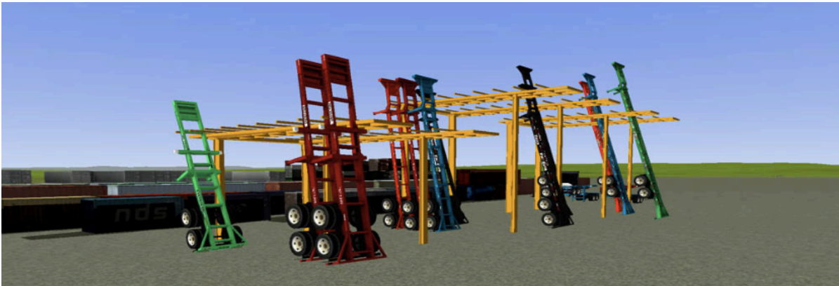
Figure Error! No text of specified style in document.-3. Example of vertical chassis storing.
