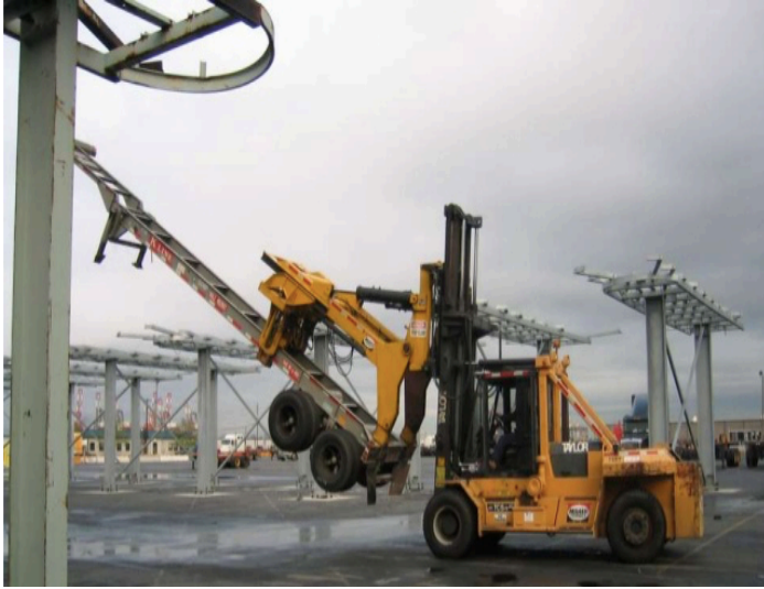
Figure Error! No text of specified style in document.-2. Specialized hydraulic stacker lifting a chassis.
