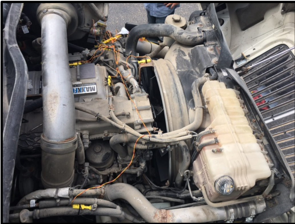
Figure 27. Overview of Under-Hood Instrumentation.
