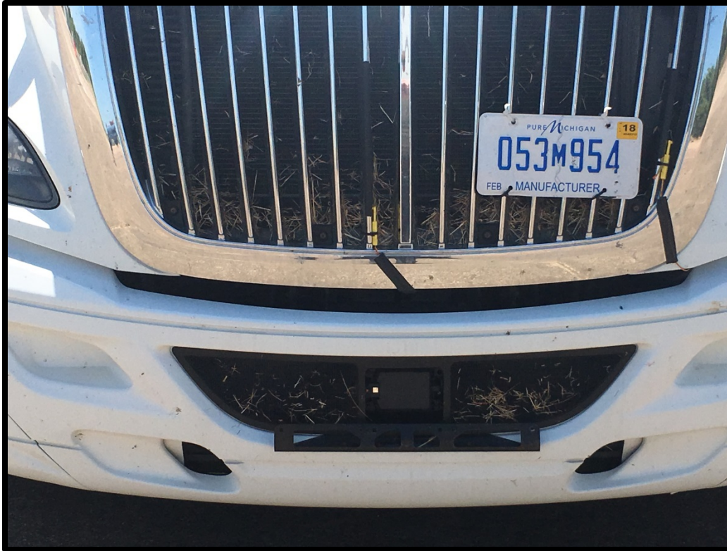
Figure 30. FV Front Grill Showing Accumulated Dirt and Debris.
