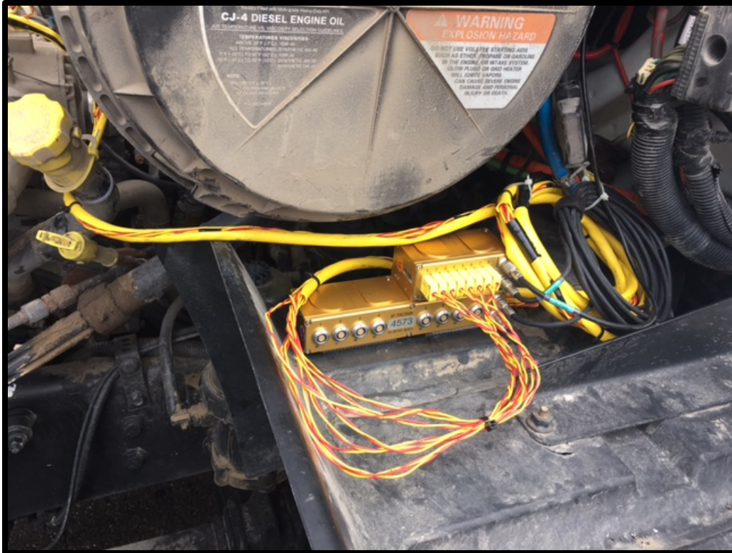
Figure 28. Thermocouple Aggregation and Logging (Open Ports Shown for Voltage/Current Sensing Shown But Not Used during Demo Event).
