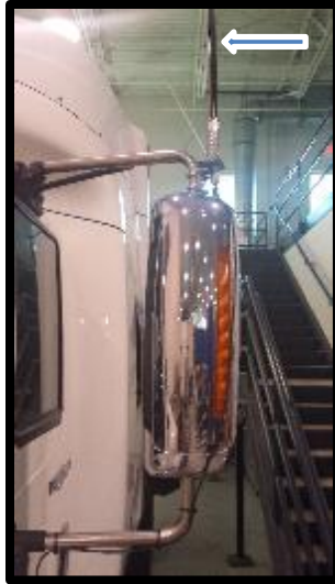
Figure 41. DSRC Antennae Installation (See Arrow).
