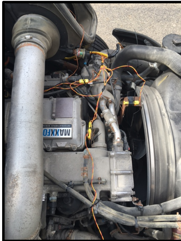
Figure 25. Fan Outlet and Intake Air Instrumentation.
