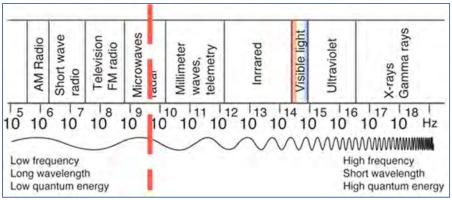
Figure 26: DSRC Frequency (53).
