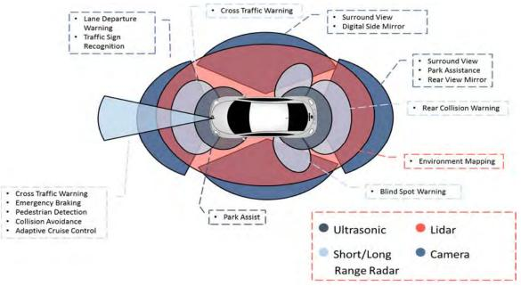
Figure 4: Menu of discrete sensor roles (4).
