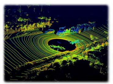
Figure 6: 64-laser LIDAR point cloud (5).
