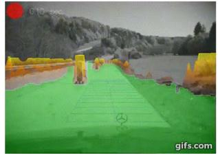
Figure 16: Grid-based Occupancy Mapping (34).
