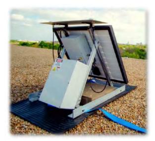
Figure 10: A stationary differential GPS unit deployed by researchers at the University of Texas (18).
