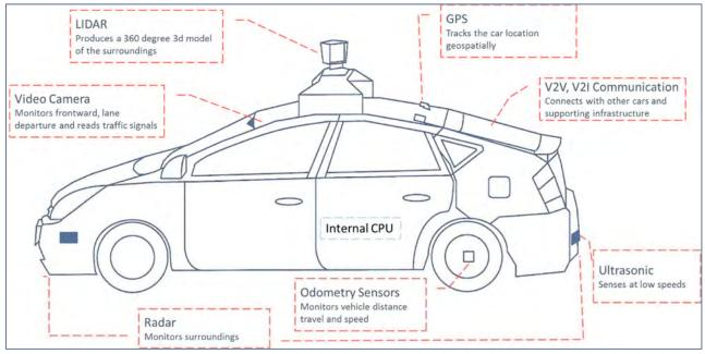
Figure 2: Autonomous Vehicle Sensor Suite (3).
