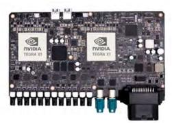
Figure 13: NVIDIA Drive PX 2 (27)
