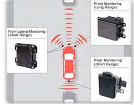
Figure 12: Radar systems in AVs (24).
