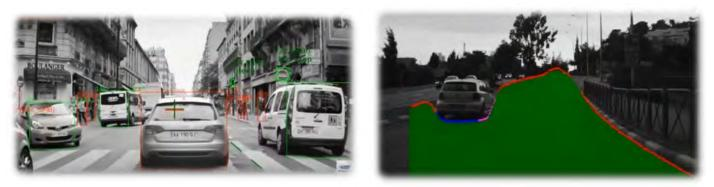
Figure 11: Camera-based object and sign detection and clear space detection (20).
