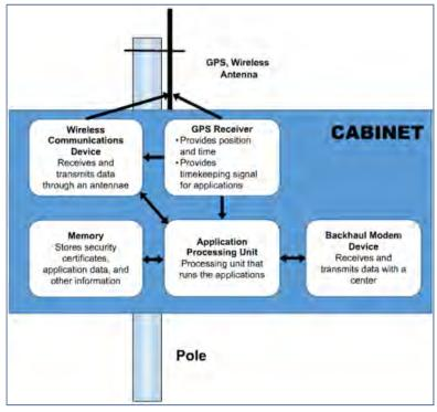
Figure 28: Overview of RSU Functions (51).
