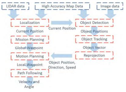
Figure 14: LIDAR Dependent Software Process(31)
