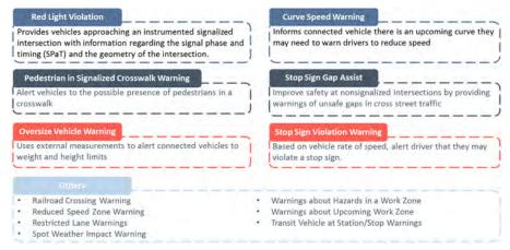
Figure 24: Potential V2I Safety Applications (51).
