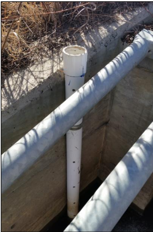
Figure 17. Levellogger™ pressure transducer installation over 2014 and 2015 rainfall seasons allowed testing of the elliptical slot weir in the field.
