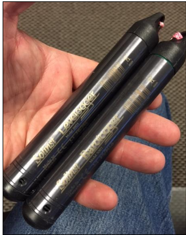
Figure 17. Levellogger™ pressure transducer installation over 2014 and 2015 rainfall seasons allowed testing of the elliptical slot weir in the field.
