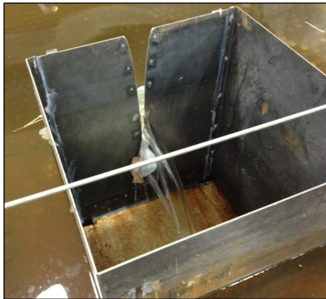
Figure 12. Qualitative observations on debris handling indicate that the elliptical slot weir handles debris better than does an orifice plate with a well screen covering the water quality orifices.
