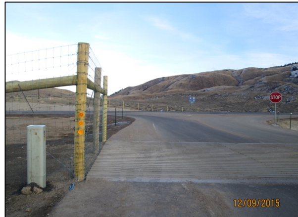
Figure 2. U-bolt system used to securely mount camera boxes to T-posts (left). Example of a camera installed inside a utility box to hide cameras in high traffic areas, such as this deer guard (right).
