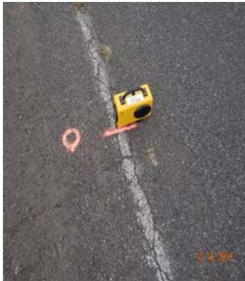
Figure 5.16: WAS Speaker Facing Sound Meter
