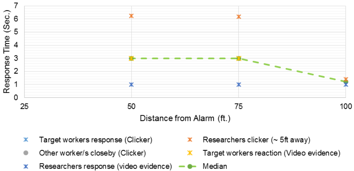
Figure F.4: Screed Operator Response Time (SonoBlaster®)
