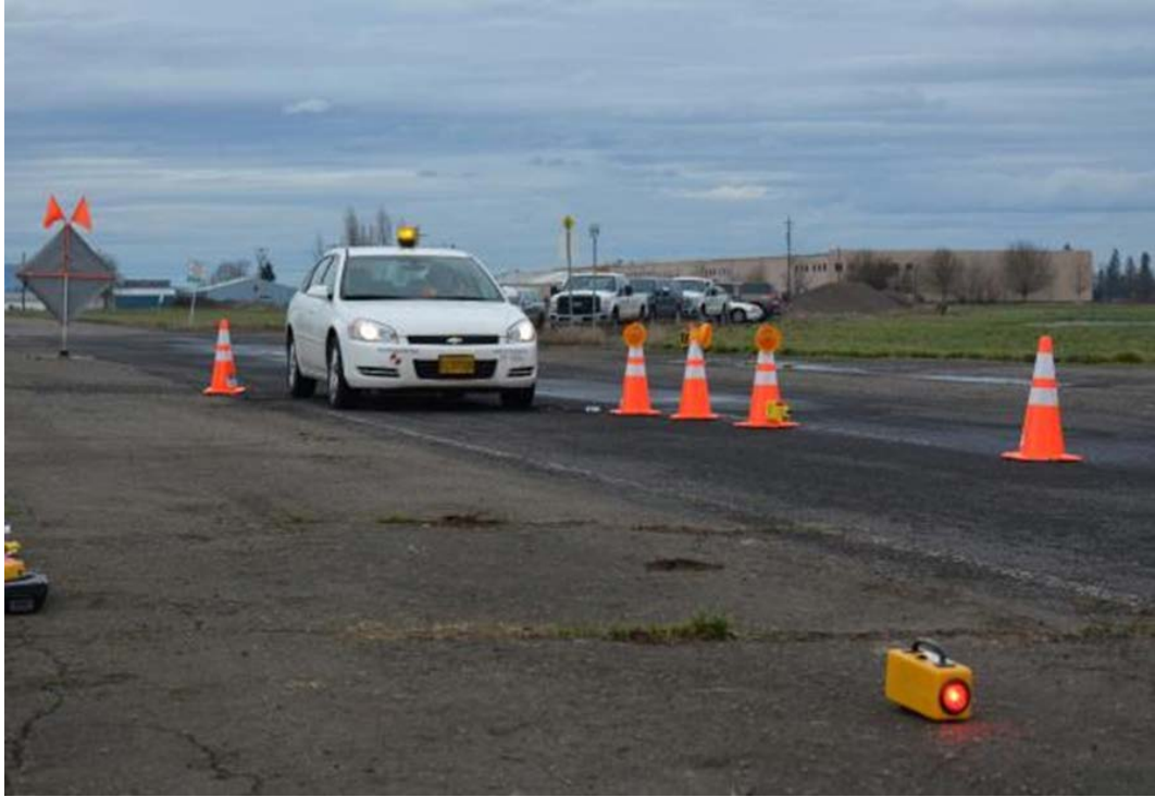
Figure 6.8: WAS Located 50ft from Equipment while Activated by Intruding Vehicle
