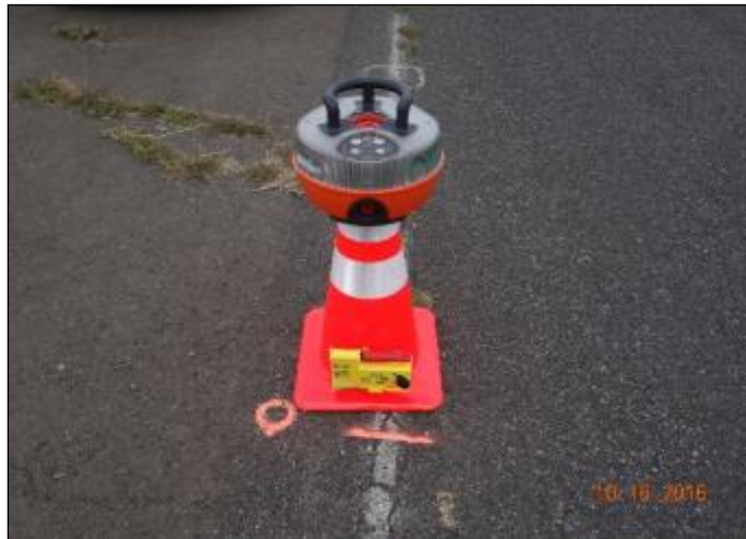
Figure 5.10: One Speaker Oriented towards Sound Meter
