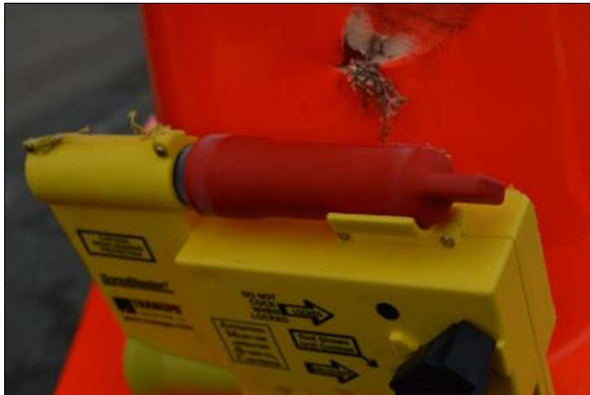
Figure 5.2: SonoBlaster® Damaged after Simulated Intrusion (Vehicle Striking Cone)
