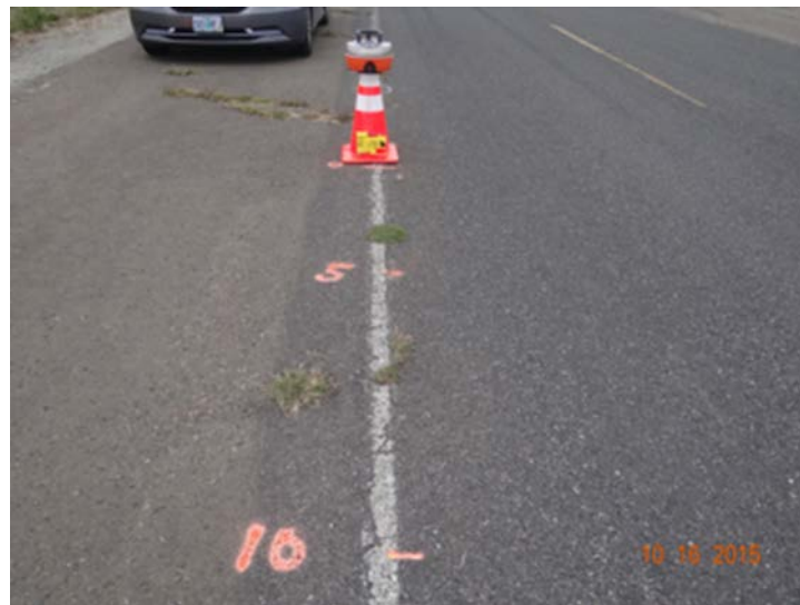
Figure 5.3: Distance Markings (in feet) on Roadway
