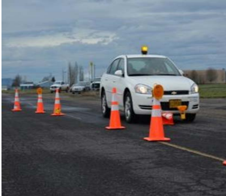
Figure 6.6: Intellicone® Activated on Impact
