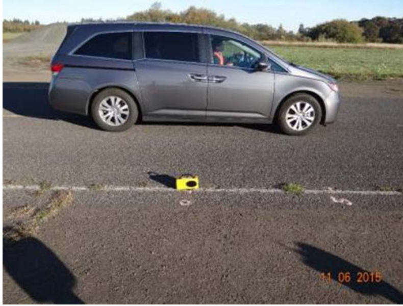
Figure 5.19: Test Setup for Sound Level Measurement inside Vehicle
