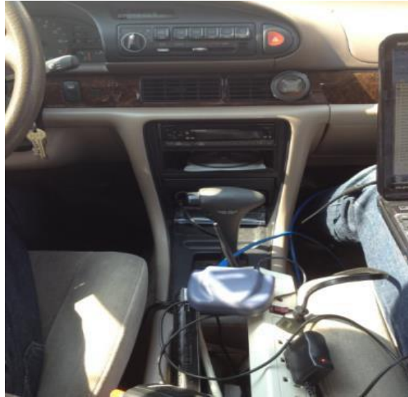
Figure 8. The RFID Receiver is Inside a Vehicle, however the Antenna of which can be Placed Inside or Outside the Vehicle, Depending on the Connection Availability.
