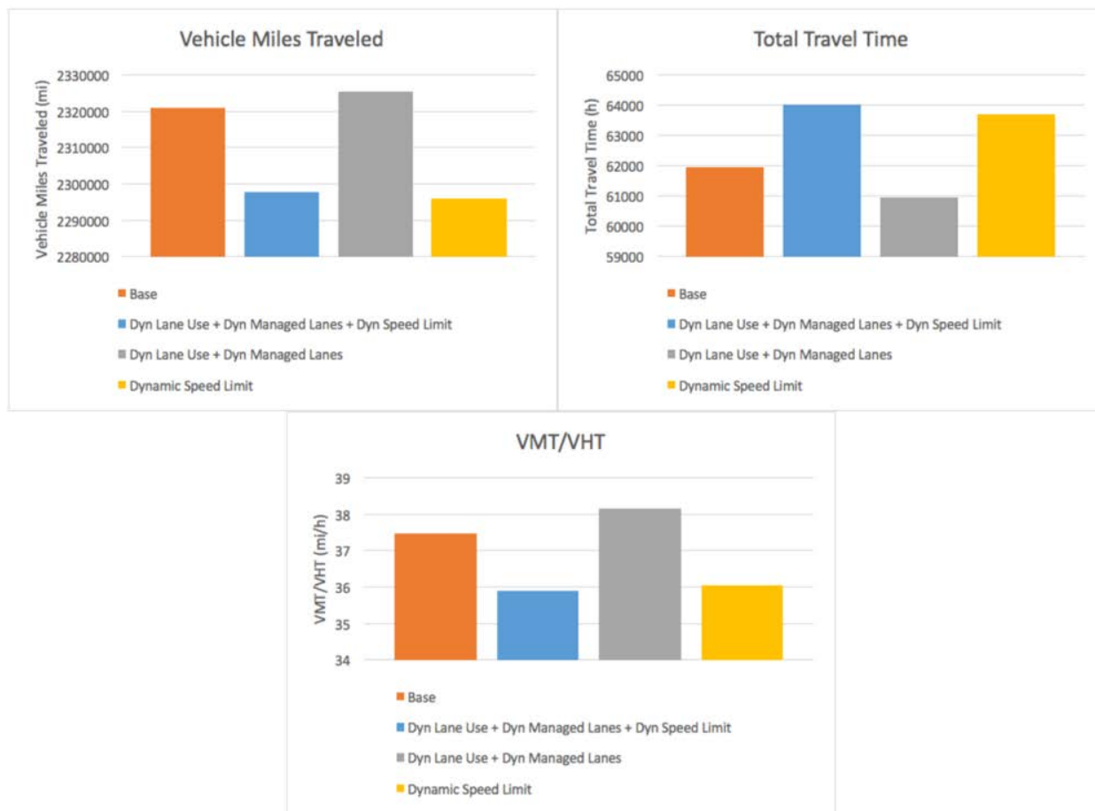
Figure 8-7: Performance measures with Dynamic Lane Use, Dynamic HOV/Managed Lanes and Dynamic Speed Limits compared with the baseline case and with the activation of individual ATDM strategies
