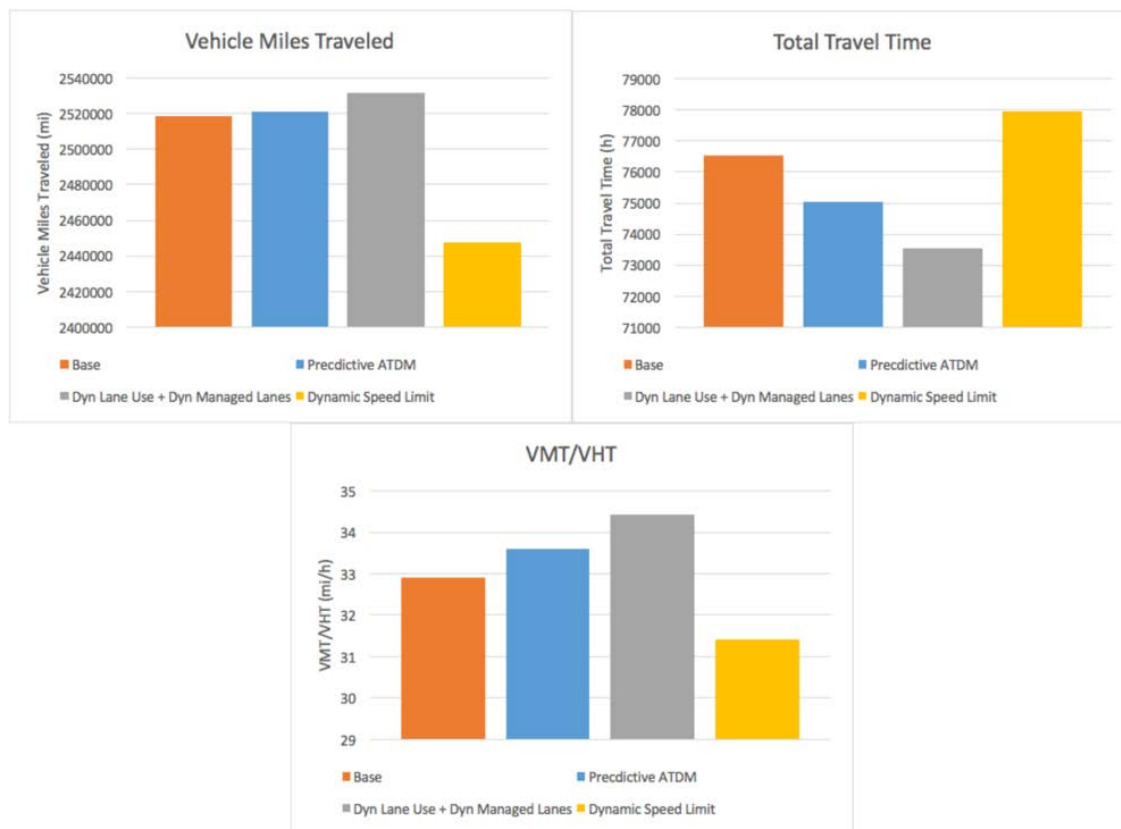
Figure 11-6: Performance measures with Predictive Traveler Information compared with the baseline case and with the activation of individual ATDM strategies under Operational Condition 3
