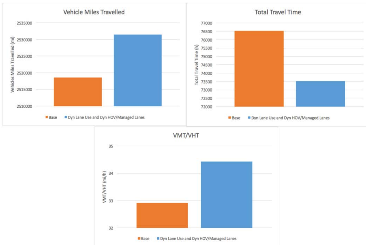
Figure 9-32: Performance measures with Dynamic Lane Use and Dynamic HOV/Managed Lanes compared with the baseline case under Operational Condition 3
