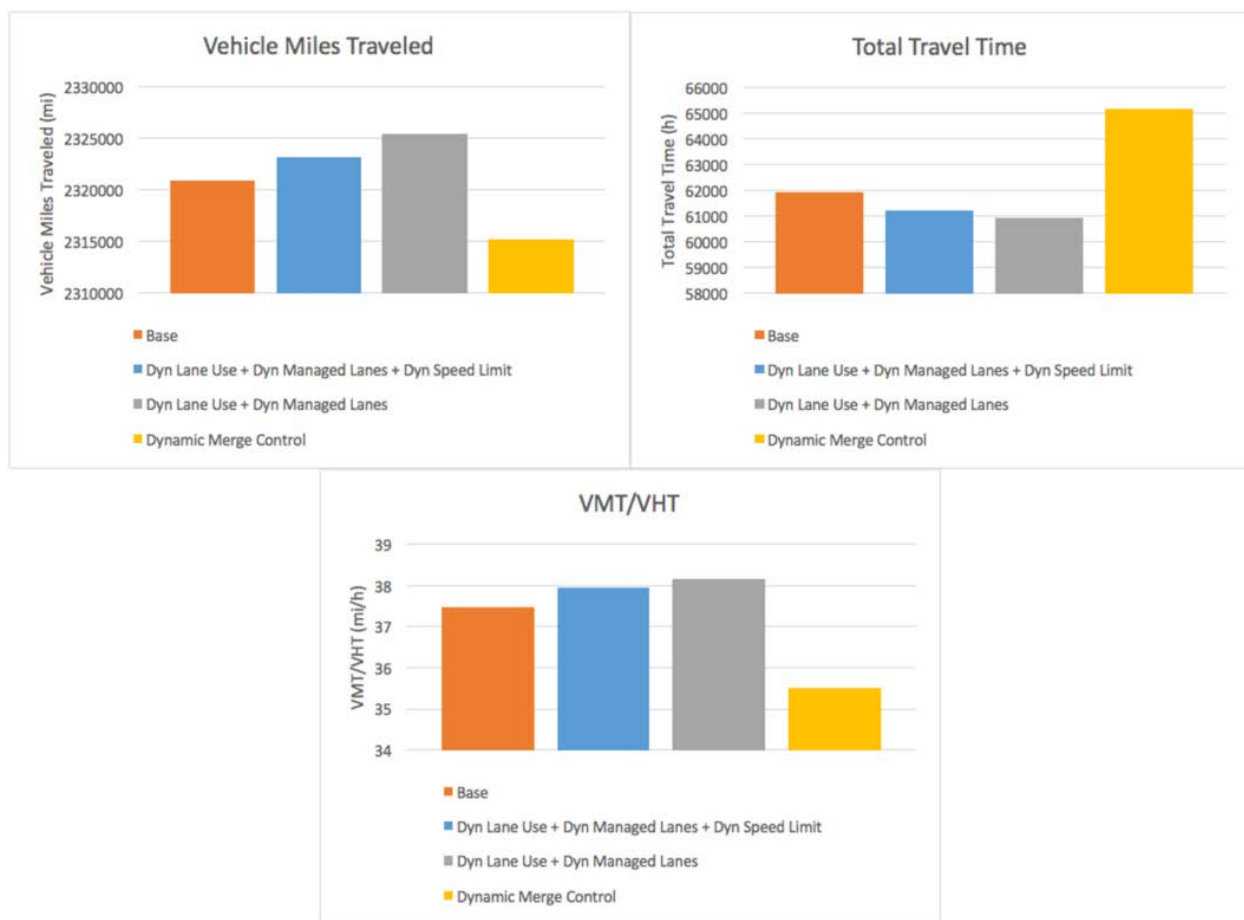
Figure 8-11: Performance measures with Dynamic Merge Control, Dynamic HOV/Managed Lanes and Dynamic Routing compared with the baseline case and with the activation of individual ATDM strategies
