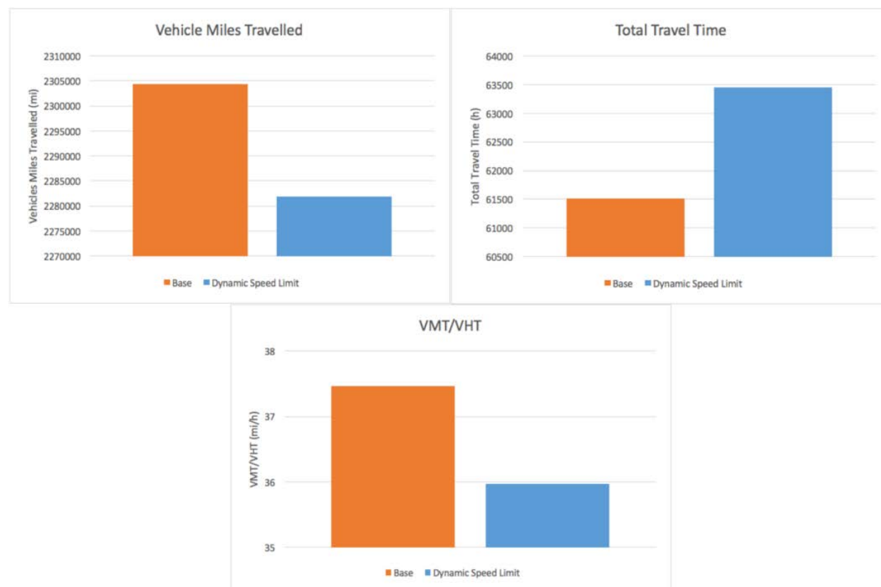
Figure 9-38: Performance measures with Dynamic Speed Limits compared with the baseline case under Operational Condition 2
