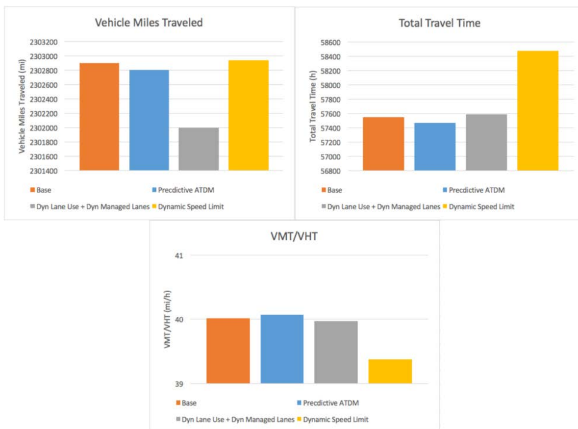
Figure 11-8: Performance measures with Predictive Traveler Information compared with the baseline case and with the activation of individual ATDM strategies under Operational Condition 4
