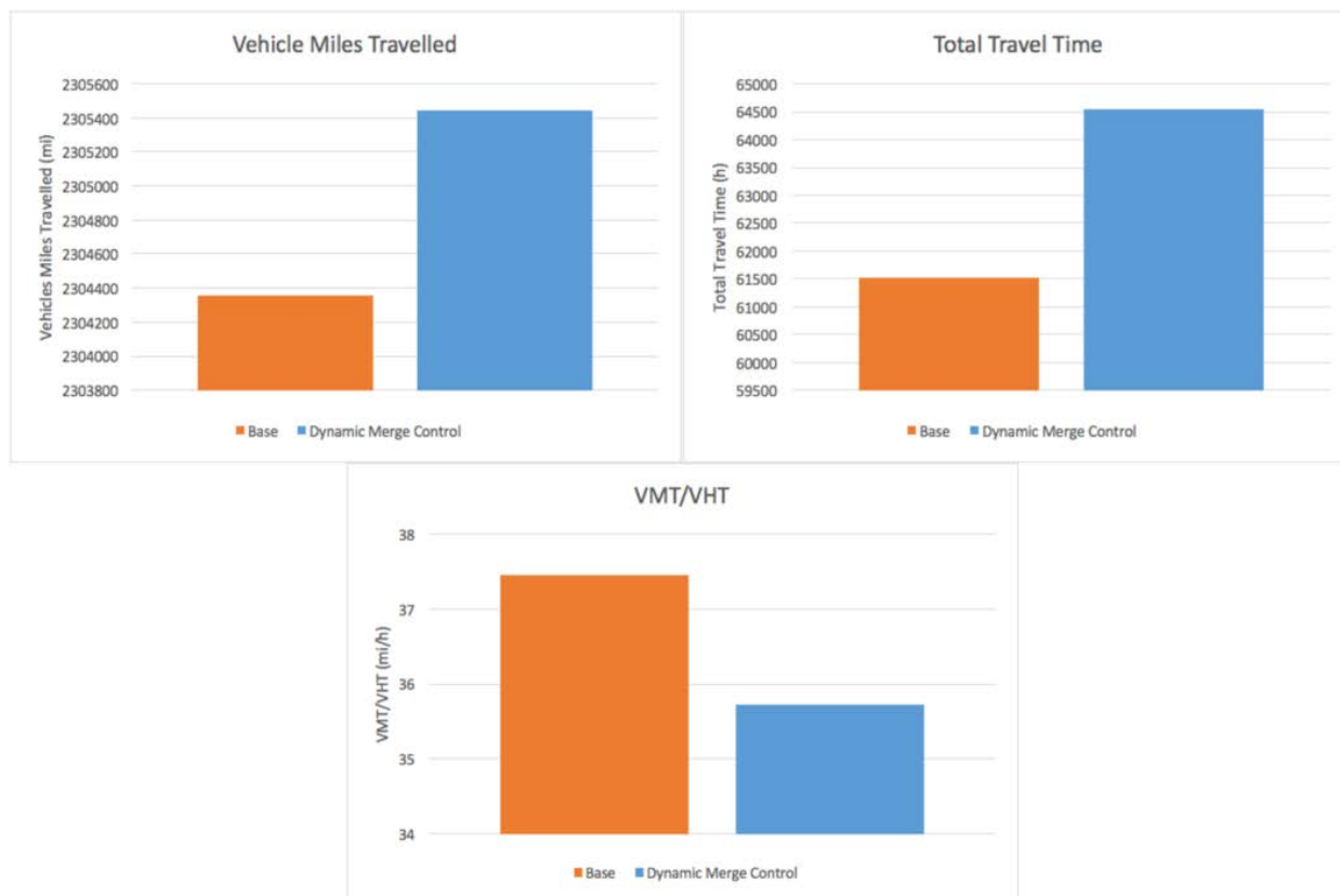
Figure 9-46: Performance measures with Dynamic Merge Control compared with the baseline case under Operational Condition 2
