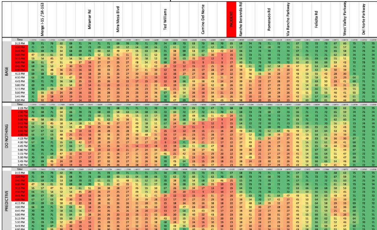
Figure 9-49: Speed contour with Predictive Traveler Information compared with the do-nothing and the baseline case under Operational Condition 3; the red boxes mark the location and the duration of the incident
