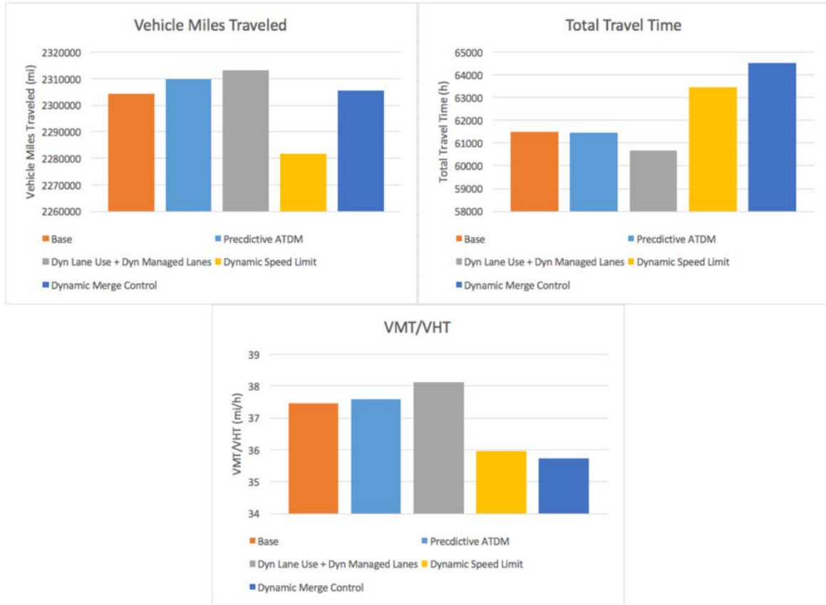
Figure 11-4: Performance measures with Predictive Traveler Information compared with the baseline case and with the activation of individual ATDM strategies under Operational Condition 2
