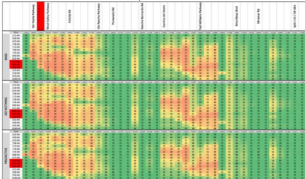
Figure 9-47: Speed contour with Predictive Traveler Information compared with the do-nothing and the baseline case under Operational Condition 1; the red boxes mark the location and duration of the incident
