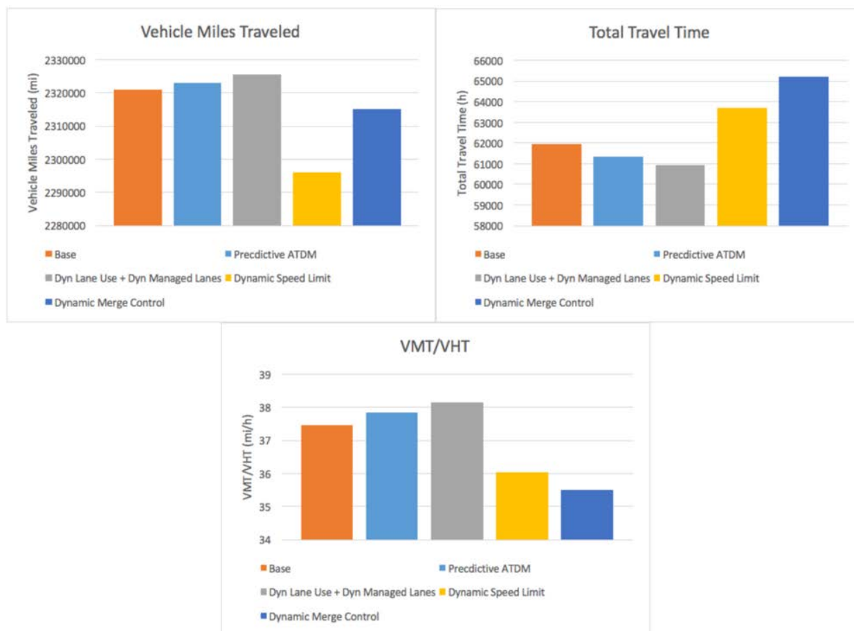
Figure 11-2: Performance measures with Predictive Traveler Information compared with the baseline case and with the activation of individual ATDM strategies under Operational Condition 1
