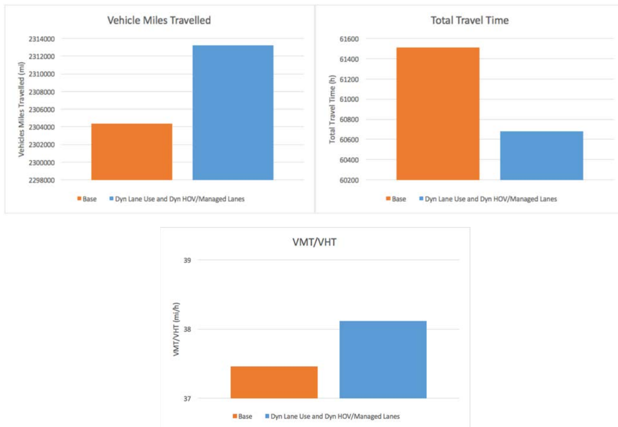
Figure 9-30: Performance measures with Dynamic Lane Use and Dynamic HOV/Managed Lanes compared with the baseline case under Operational Condition 2
