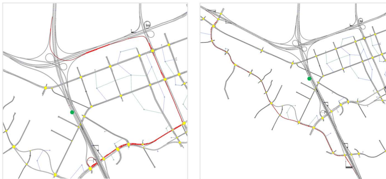
Figure 7-3: The two rerouting options for Operational Condition 1
