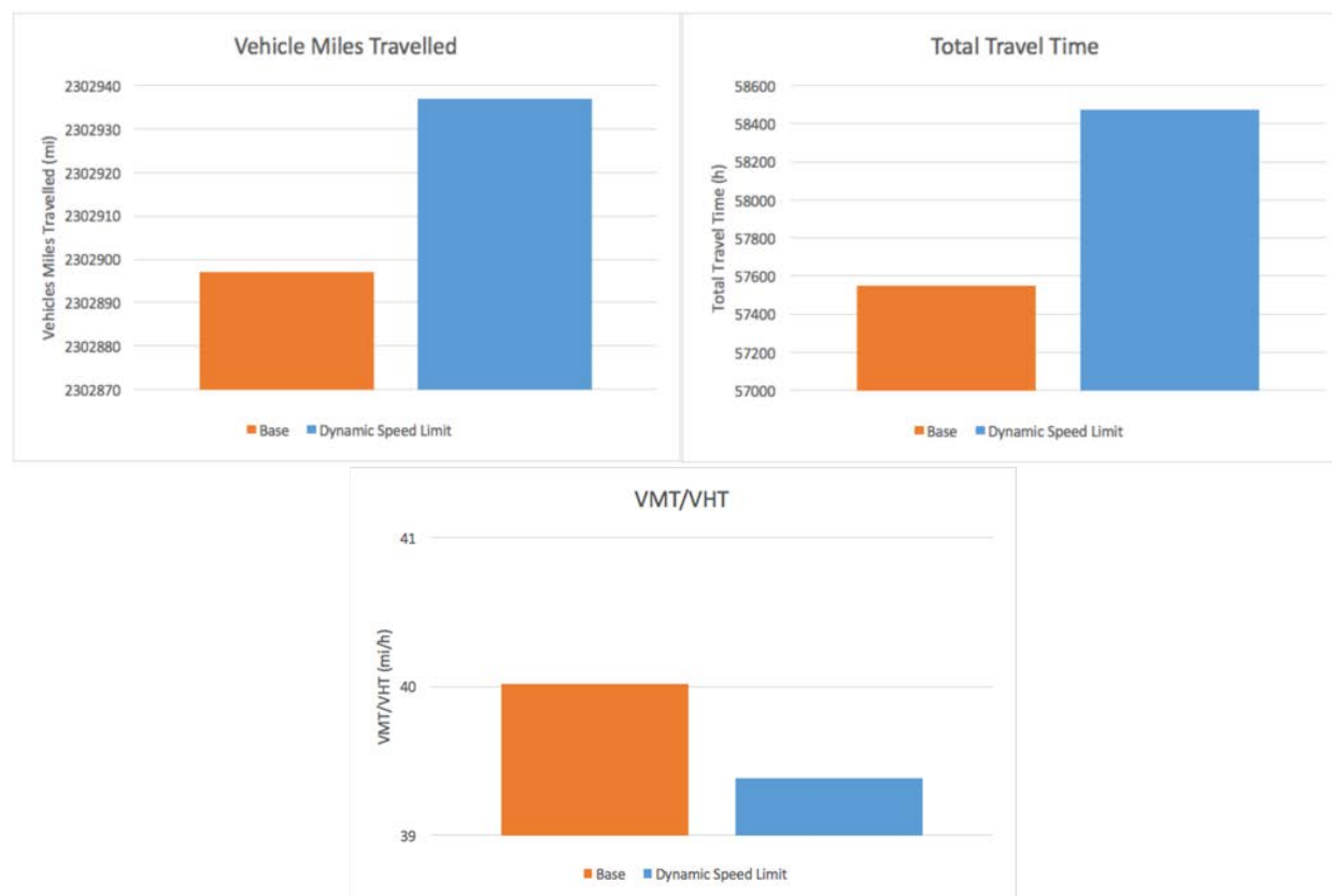
Figure 9-42: Performance measures with Dynamic Speed Limits compared with the baseline case under Operational Condition 4
