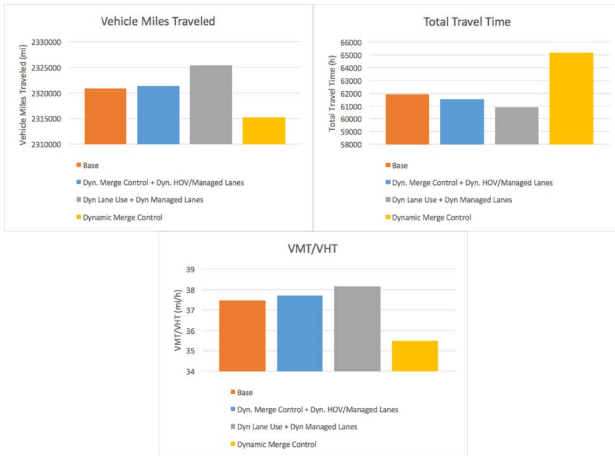
Figure 8-9: Performance measures with Dynamic Merge Control and Dynamic HOV/Managed Lanes compared with the baseline case and with the activation of individual ATDM strategies
