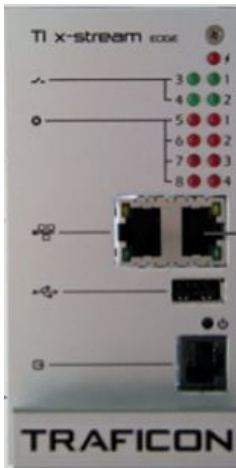
Figure 5-39. The TI X-Stream is the Single Board Computer that controls and powers the TrafiSense cameras.
