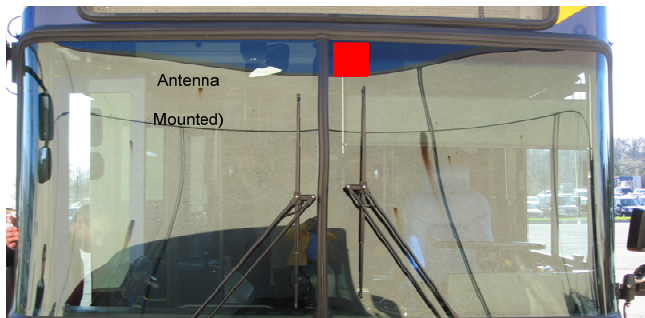
Figure 5-8. DSRC Antenna Mounting Location
