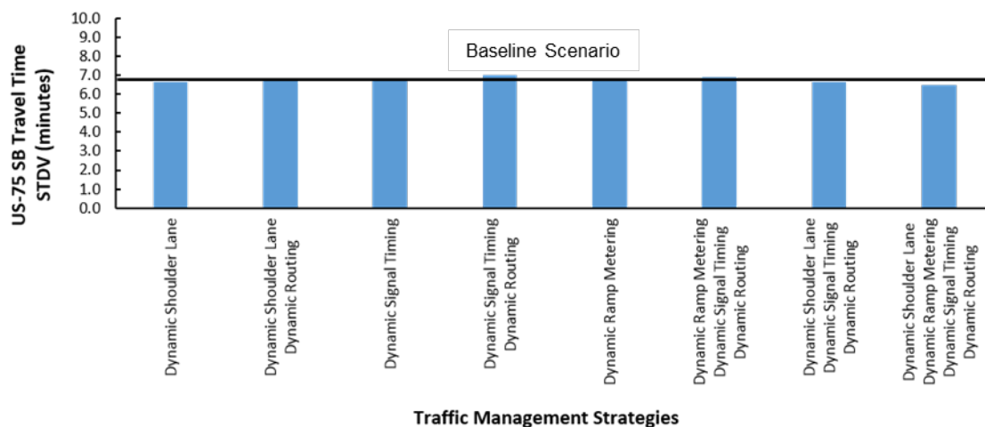
Figure 5-6: US-75 Southbound Travel Time Standard Deviation under different Traffic Management Strategies (Dallas Testbed under Medium Demand and Low Incident Severity Conditions) [Source: SMU]
