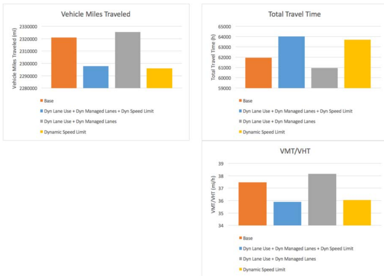
Figure 5-21: Performance measures with Dynamic Lane Use, Dynamic HOV/Managed Lanes and Dynamic Speed Limits compared with the baseline case and with the activation of individual ATDM strategies [Source: TSS]
