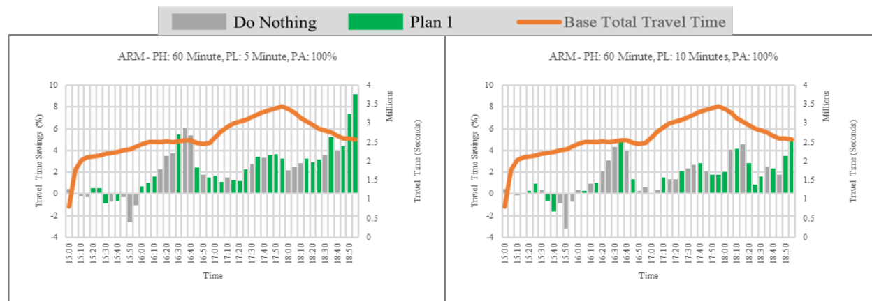
Figure 8-7: Effects of Prediction Latency on ARM Network Travel Time Savings [Source: Booz Allen]
