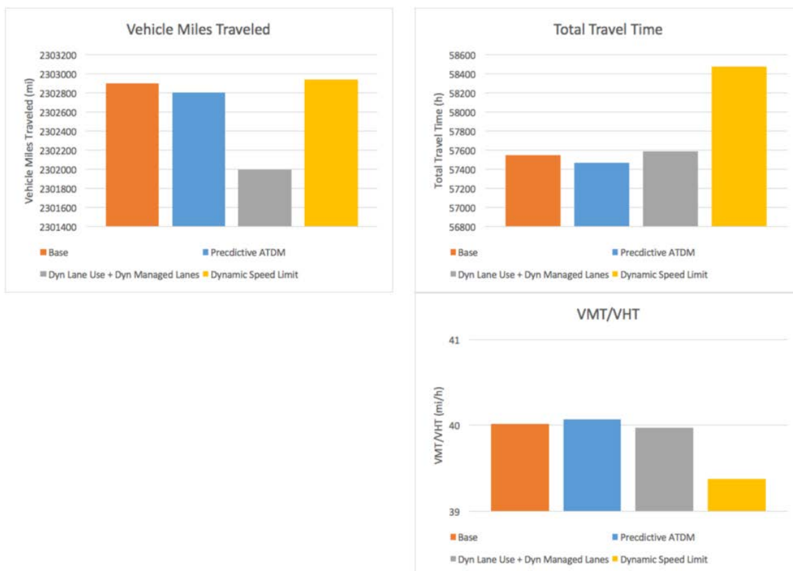
Figure 6-36: Performance measures with Predictive Traveler Information compared with the baseline case and with the activation of individual ATDM strategies under Operational Condition 4 [Source: TSS]
