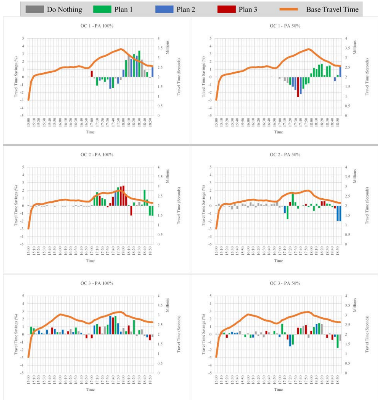
Figure 7-29: Effects of Prediction Accuracy on DSC Network Travel Time Savings under Different Operational Conditions [Source: Booz Allen]
