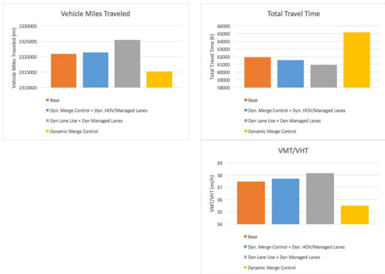
Figure 5-23: Performance measures with Dynamic Merge Control and Dynamic HOV/Managed Lanes compared with the baseline case and with the activation of individual ATDM strategies [Source: TSS]
