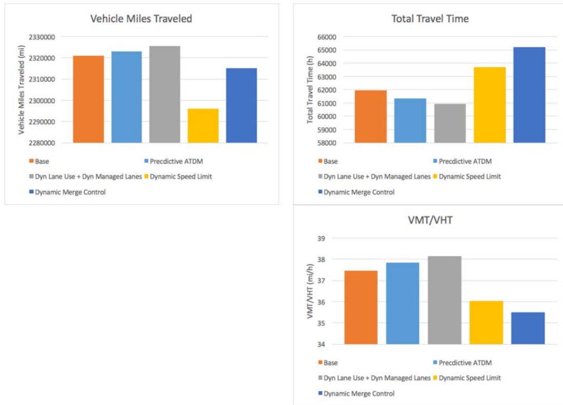
Figure 6-30: Performance measures with Predictive Traveler Information compared with the baseline case and with the activation of individual ATDM strategies under Operational Condition 1 [Source: TSS]
