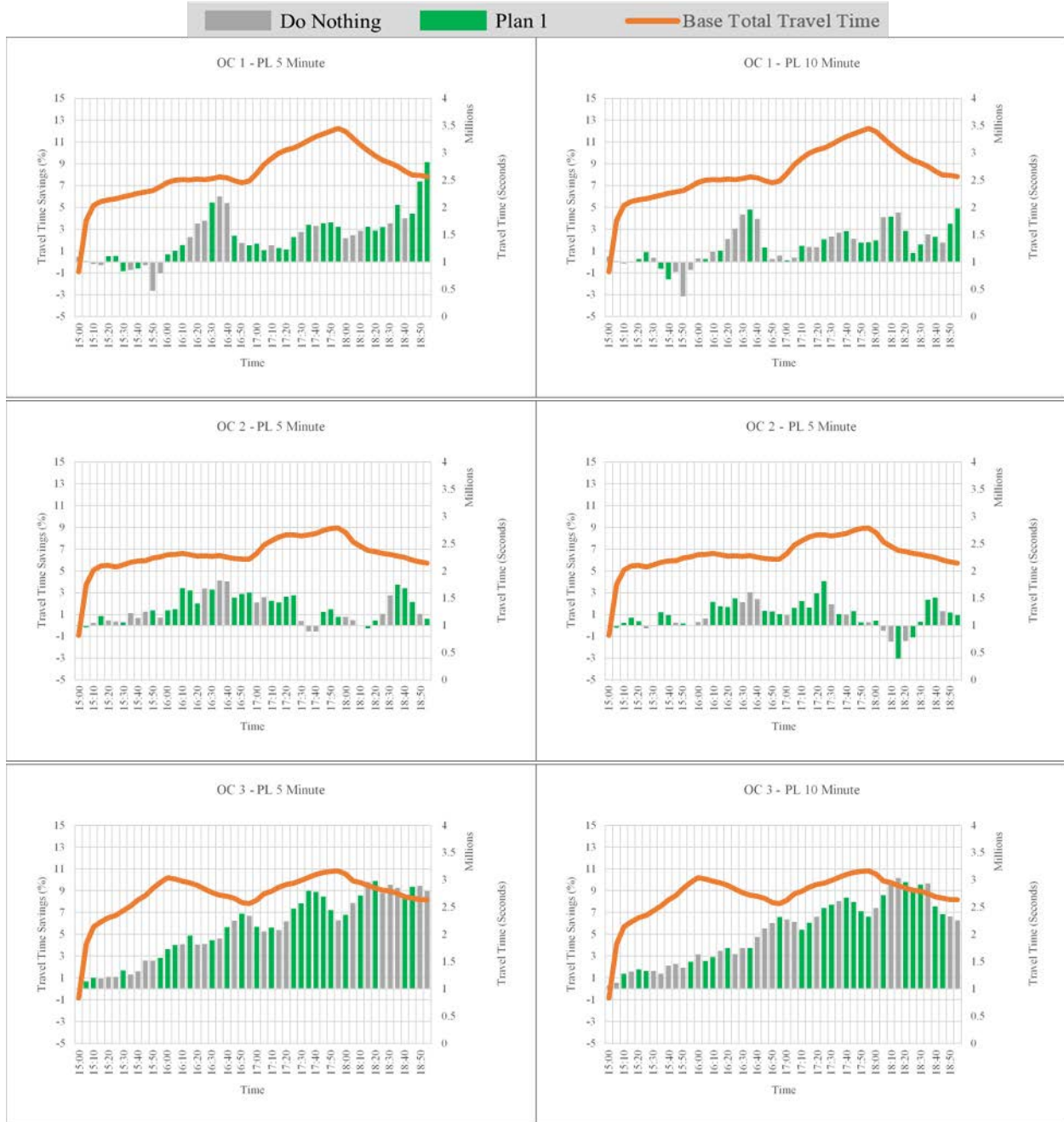
Figure 7-27: Effects of Prediction Latency on ARM Network Travel Time Savings under Different Operational Conditions [Source: Booz Allen]
