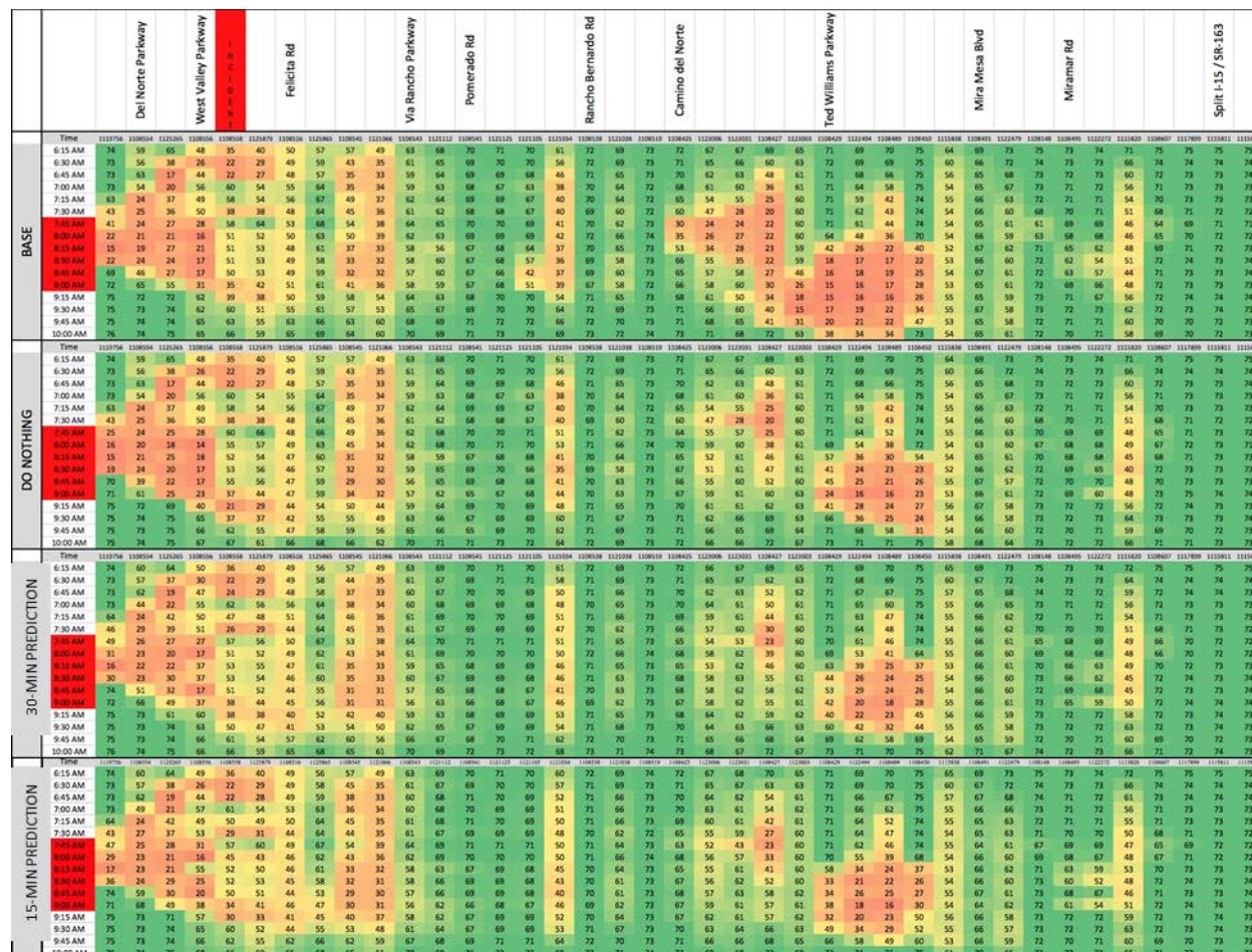
Figure 7-62: Speed contour with Predictive Traveler Information compared with the do-nothing and the baseline case under Operational Condition 2 [Source: TSS]
