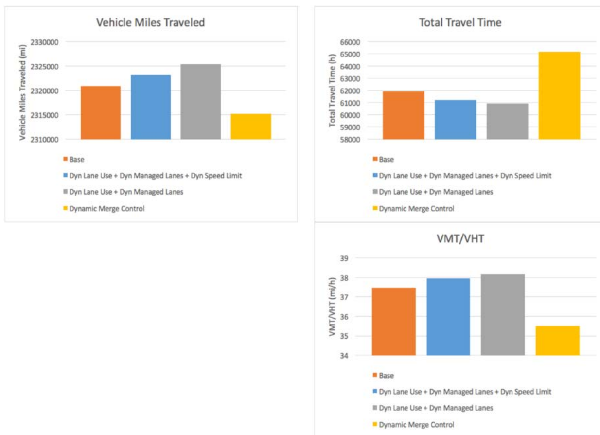
Figure 5-25: Performance measures with Dynamic Merge Control, Dynamic HOV/Managed Lanes and Dynamic Routing compared with the baseline case and with the activation of individual ATDM strategies [Source: TSS]
