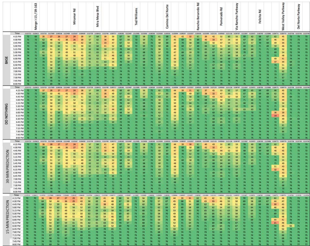
Figure 7-64: Speed contour with Predictive Traveler Information compared with the do-nothing and the baseline case under Operational Condition 4 [Source: TSS]
