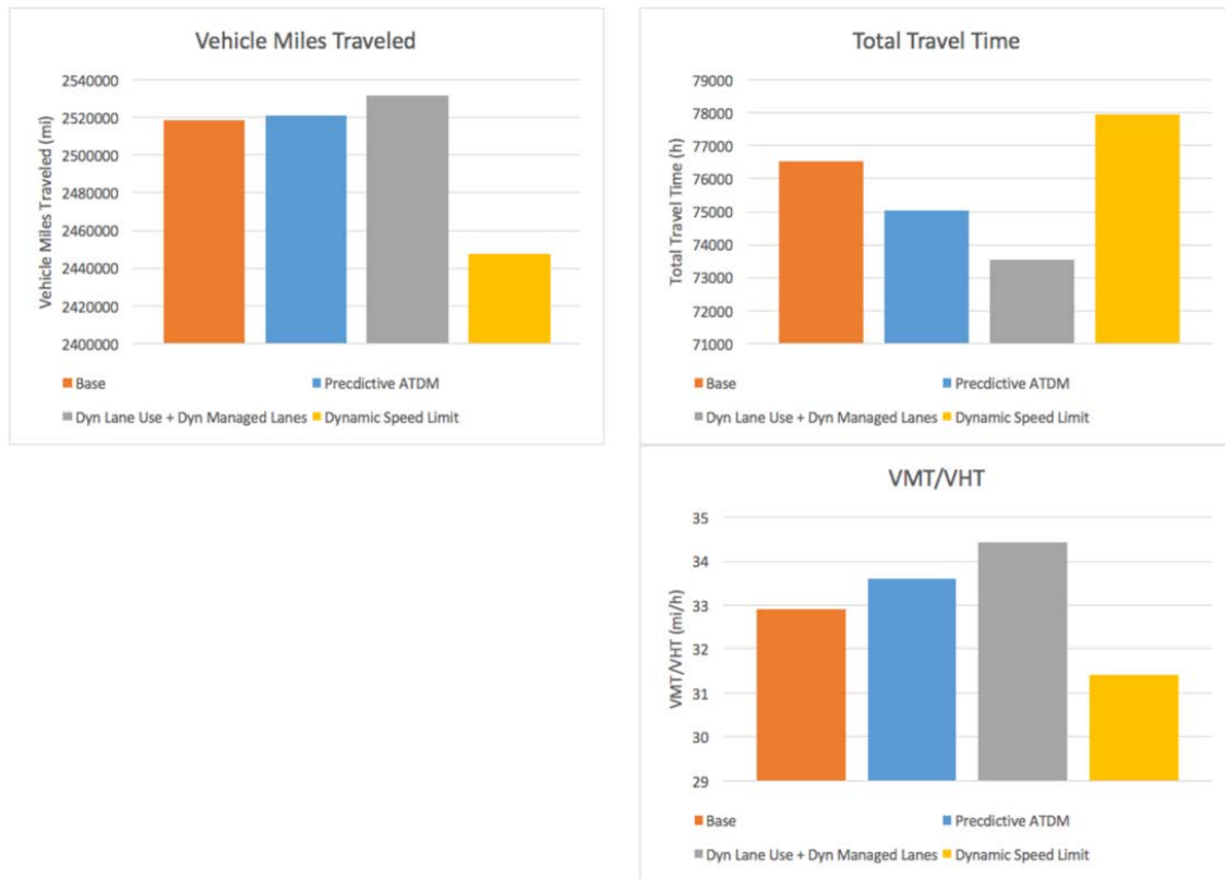
Figure 6-34: Performance measures with Predictive Traveler Information compared with the baseline case and with the activation of individual ATDM strategies under Operational Condition 3 [Source: TSS]
