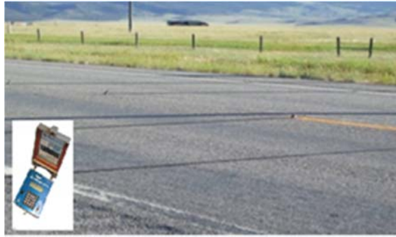
Figure 2: Typical Vehicle Classification Road Tube Setup (Wuertley and Little 2013)
