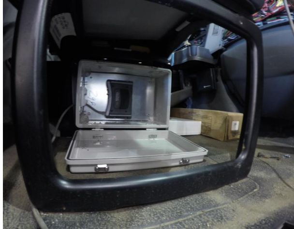
Figure A.4: Modem Mounted under the Passenger Seat Inside of Enclosure.
