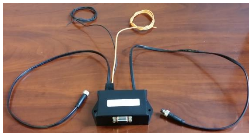
Figure A.9: RoadWatch SS DE-9 (DB-9, or RS-232) Converter Box.
