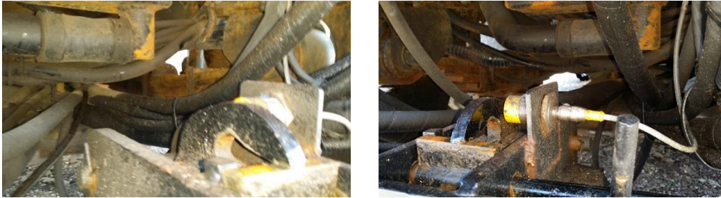
Figure A.26: Sensor and Plow Hook in the “Plow Off” Position.
