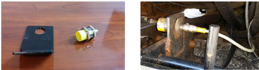
Figure A.10: Unmodified Mounting Bracket and Proximity Sensor (left). Proximity Sensor Mounted on Modified Bracket.
