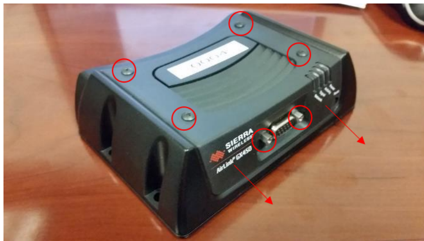
Figure D.4: Opening Procedure for GX450 Modem
