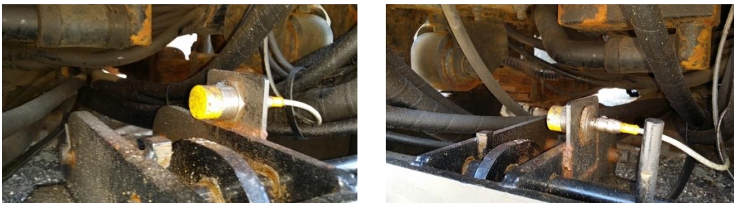
Figure A.25: Sensor and Plow Hook in the “Plow On” Position.
