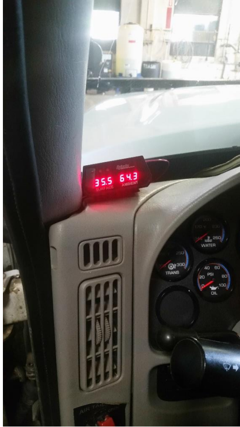
Figure 4.13: Road Temperature Sensor Display Installed in ODOT Truck.
