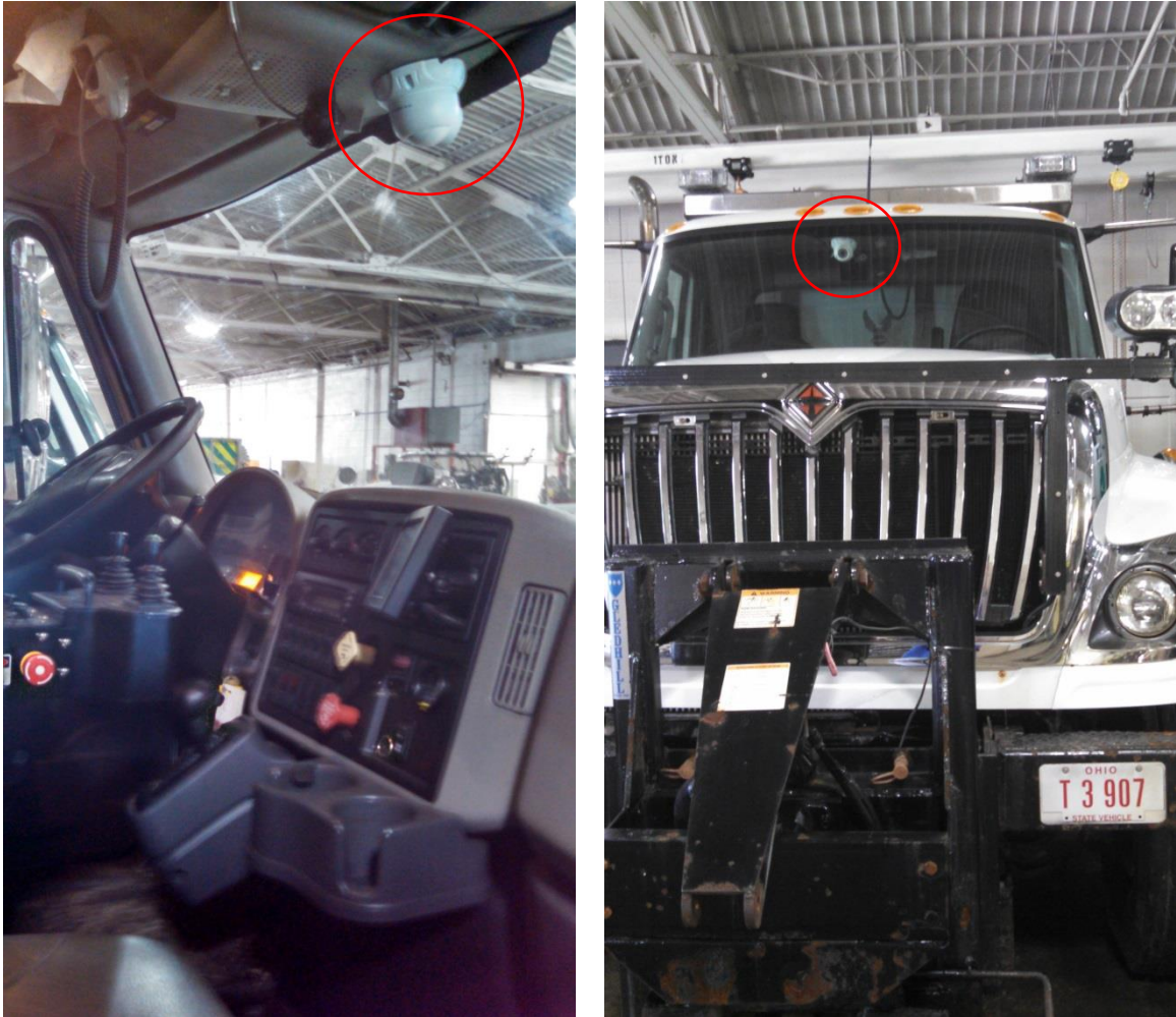
Figure A.20: Ethernet Camera Installed as Seen from in the Cab (left) and from in Front of the Vehicle (right).
