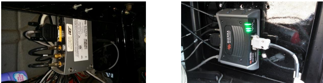
Figure A.3: Sierra Wireless GX 440 Mounted to the Back of Passenger Seat (left) and Mounted to the Door Side of the Passenger Seat (right).
