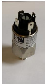
Figure A.24: Top of hydraulic pressure sensor. Note the set screw at the top.
