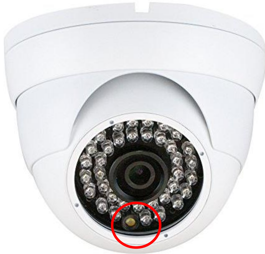
Figure A.21: Face of Ethernet Camera. Note the infrared receiver at the bottom of the camera face. Image courtesy of MicroSeven.
