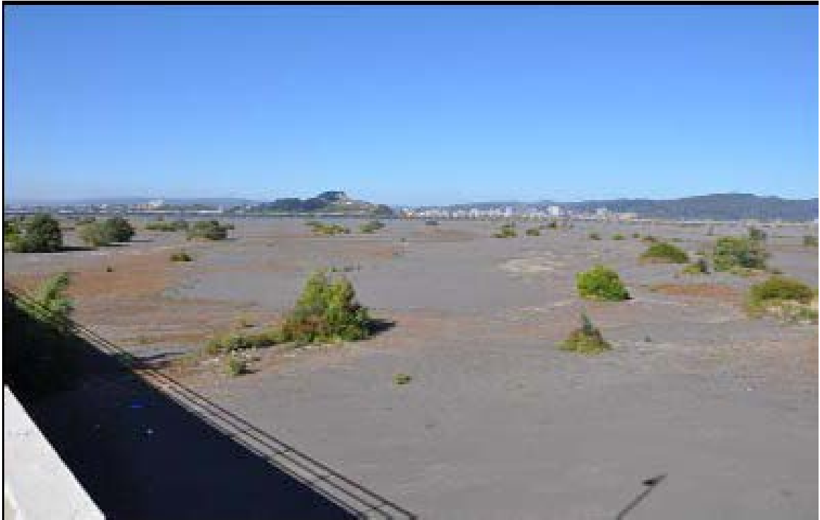
Figure 3.9. Fine-grained material brought to the surface at Juan Pablo II Bridge (Bray and Frost 2010).
